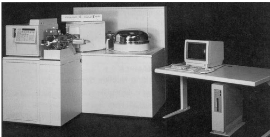
FIGURE A.2 Mass spectrophotometer. This instrument measures the mass of atoms and molecules.
