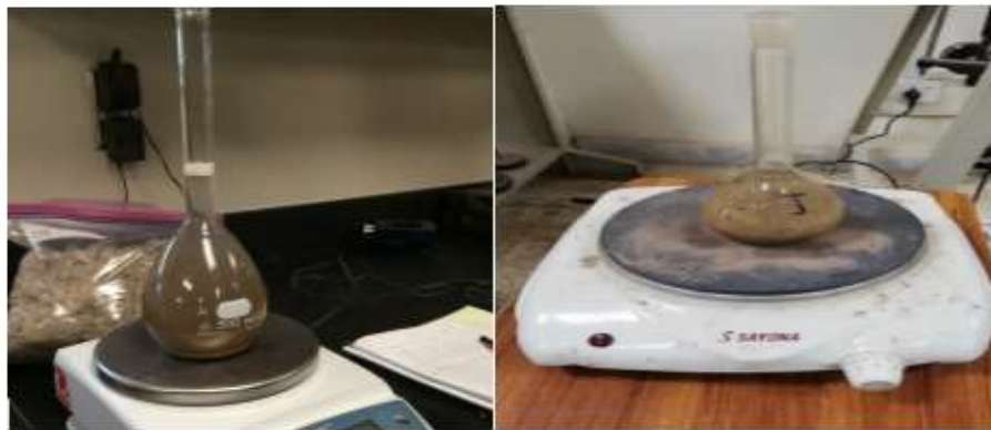
Figure 3.6: Specific gravity test was in progress
