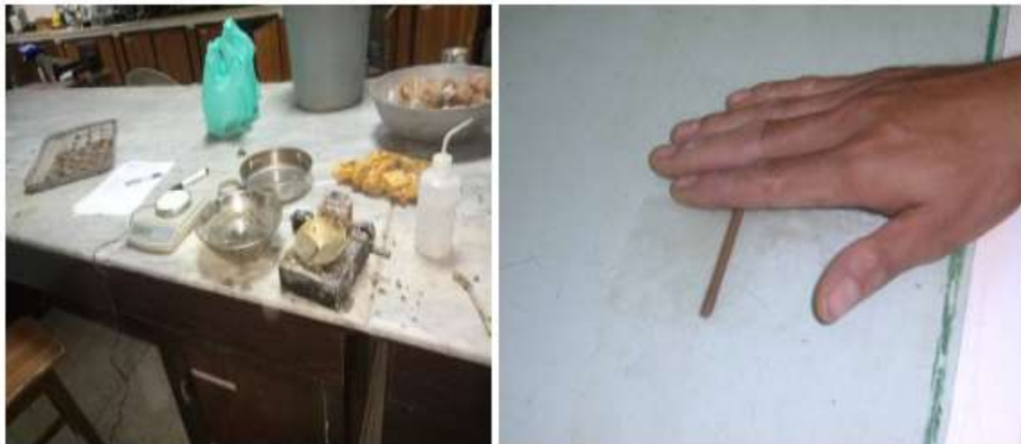
Figure 3.4: Liquid limit and Plastic limit test arrangement in laboratory
