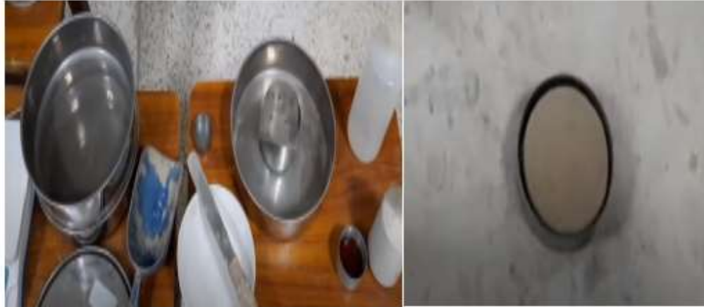
Figure 3.5: Shrinkage limit was in progress
