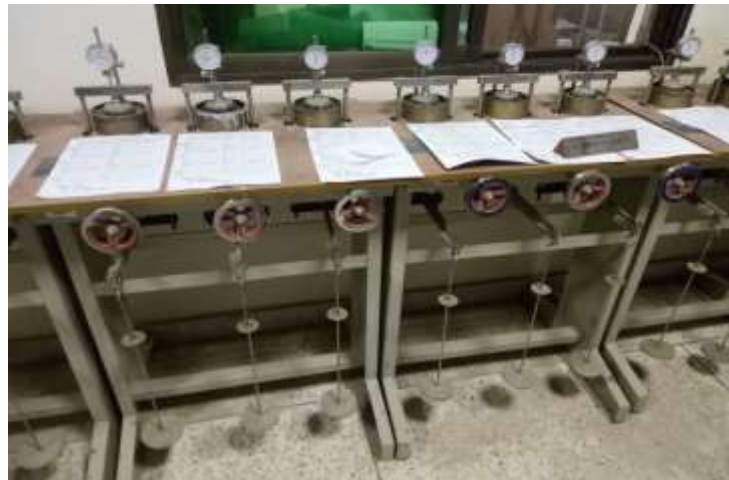
Figure 3.8: Consolidation tests were in progress
