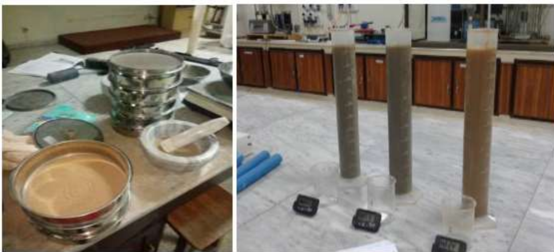
Figure 3.3: Scheme of sieve analysis and hydrometer in the laboratory
