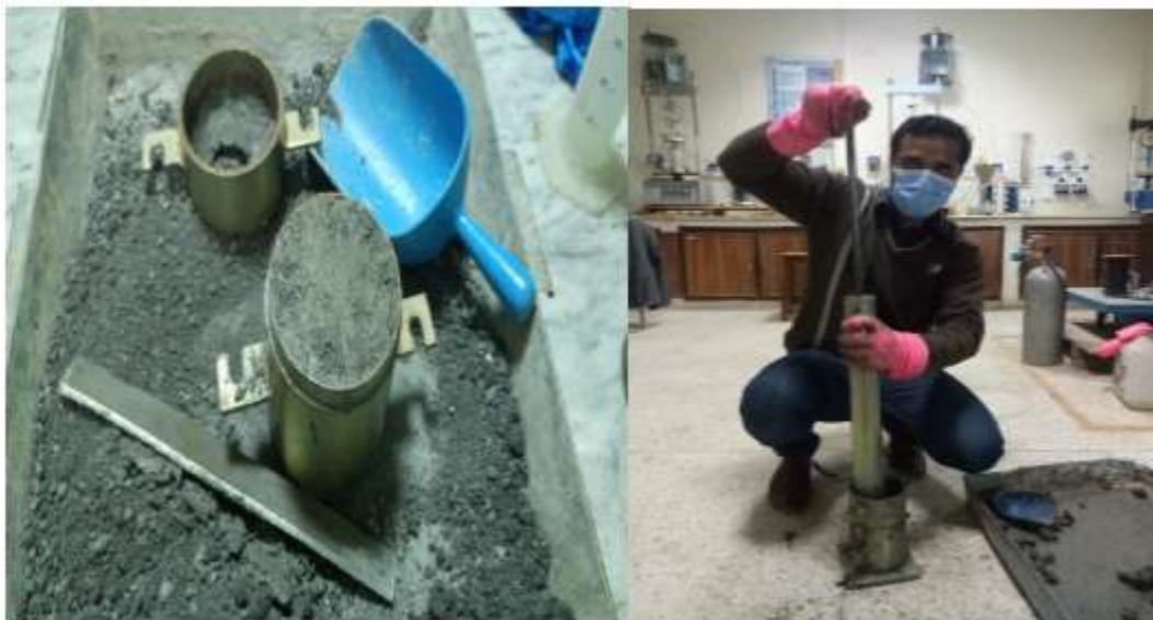
Figure 3.7: Compaction test pictorial views
