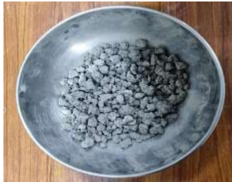
Figure 3.2: Soil sample for natural moisture content determination
