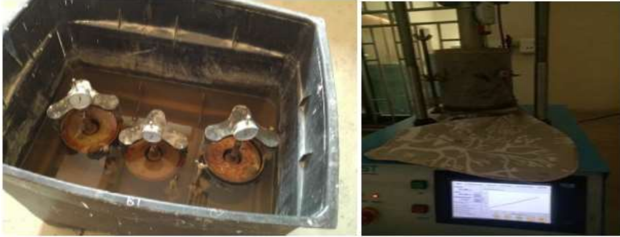
Figure 3.10: Pictorial views of the California Bearing Ratio test
