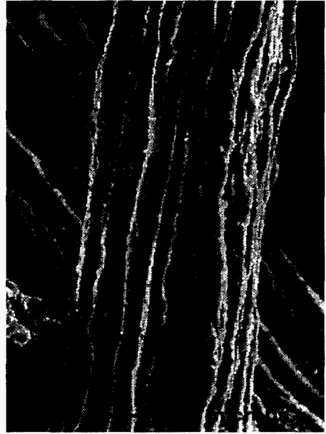
Figure 4. Scanning electron micrograph of extruded stainless steel matrix material.
