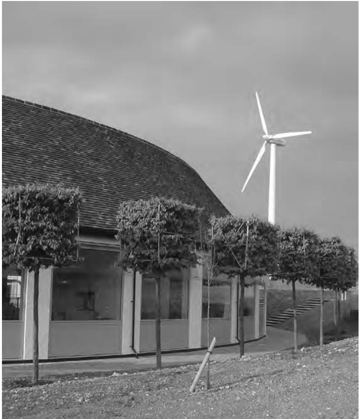
17.2 Boxed hornbeams provide solar shading.
