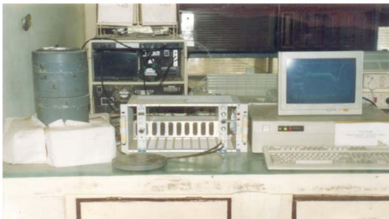
Fig. 3 NaI (Tl) gamma-ray detector coupled to a 4 K MCA
