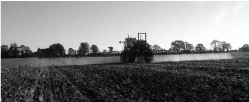
Fig. 3.2 Tractor sprayer: (a) Mounted on 3-point linkage; (b) trailed; (c, d) self-propelled with part (d) showing wide boom (24 m). ( Continued. )
