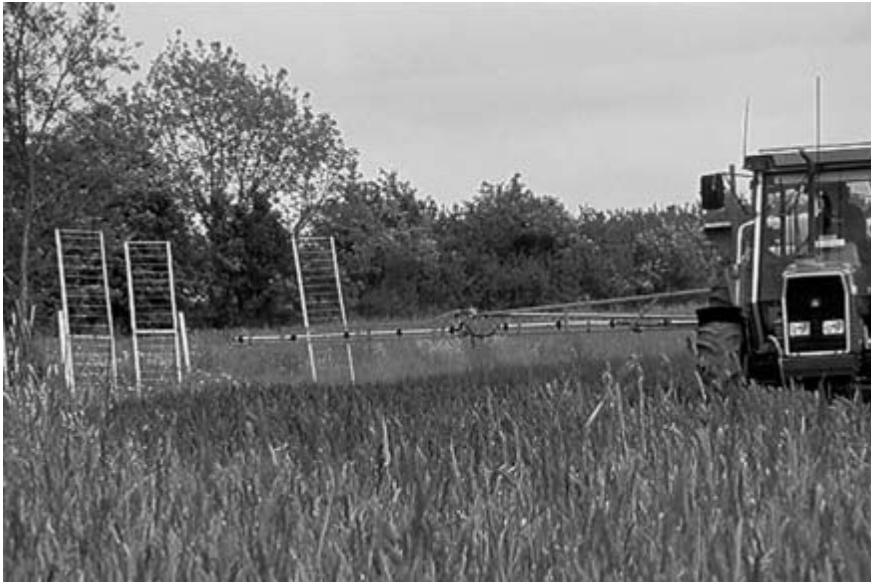
Fig. 6.13 Measuring drift adjacent to a hedgerow (courtesy Paul Miller, Silsoe Research Institute).
