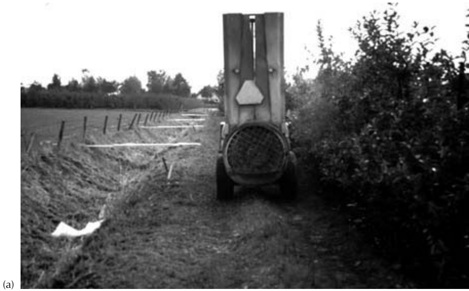
Fig. 6.2 (a) Measuring drift into a ditch. (Continued.)
