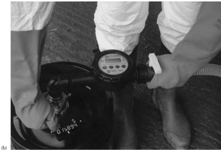
Fig. 4.6 Closed-transfer system. (a) Showing drum connected to sprayer. (b) Close up of drum with operator attaching it to sprayer.
