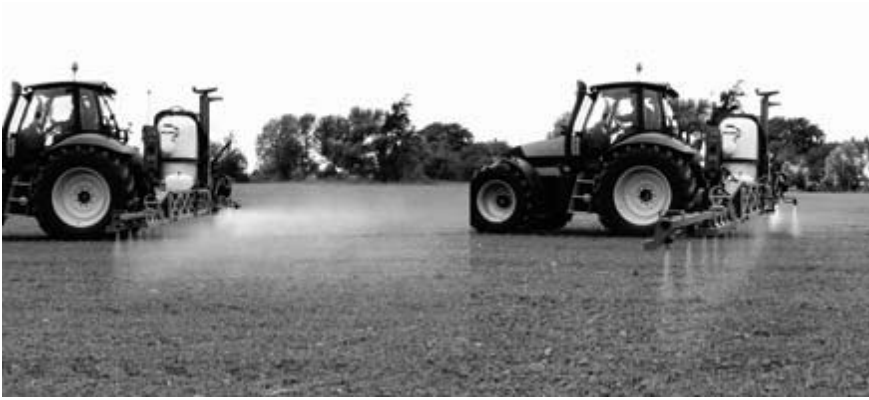
Fig. 6.6 Changing the nozzle or reducing pressure to reduce drift (photograph Hardi International).
