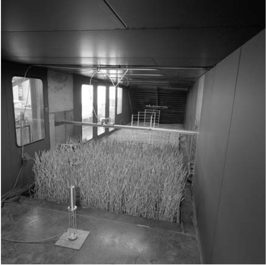
Fig. 5.3 Measuring potential drift under wind-tunnel conditions (Silsoe Research Institute).
