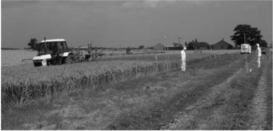
Fig. 5.6 Using a coloured dye to measure exposure to bystanders at two distances downwind of the end of the spray boom (photograph CSL).
