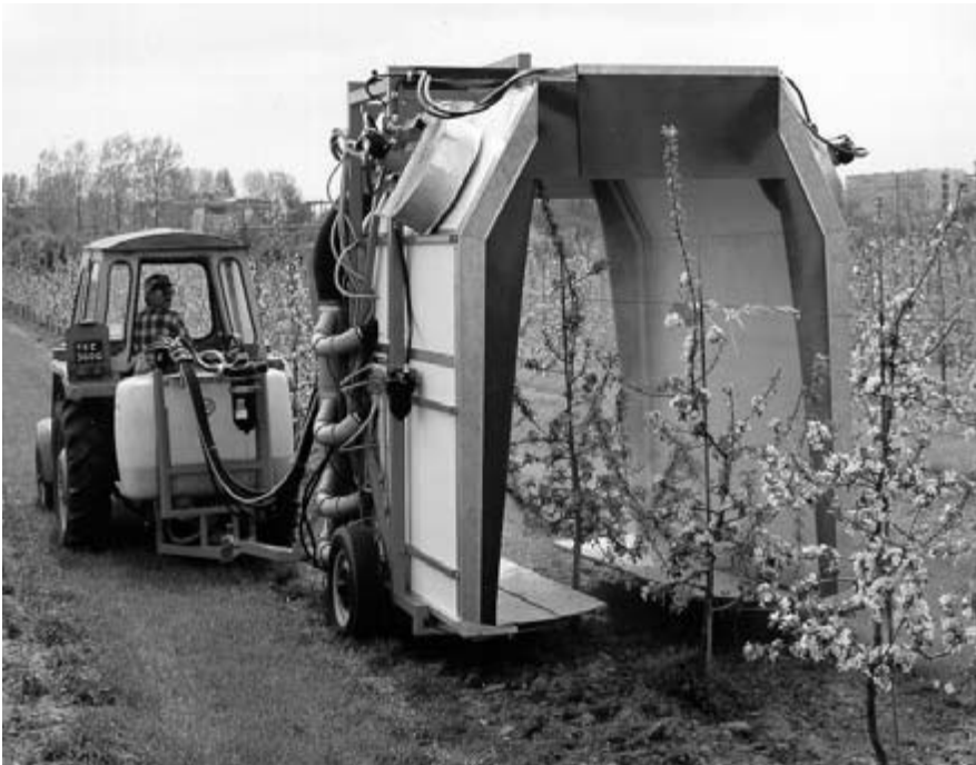
Fig. 6.9 Tunnel sprayer enclosing nozzles to reduce drift (a) in vines and (b) in apples (photograph from Greg Doruchowski, Poland).
