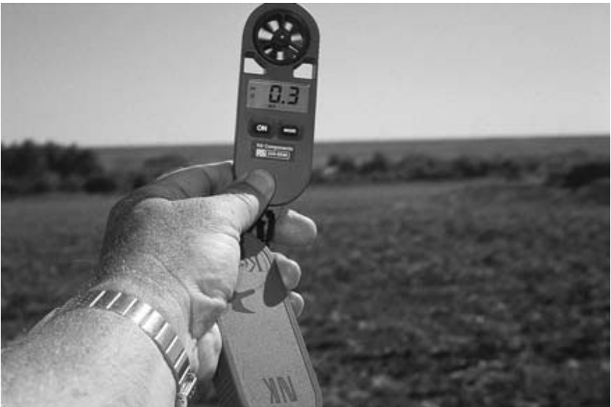
Fig. 6.5 Checking wind speed as to suitability for spraying (photograph Hardi International).
