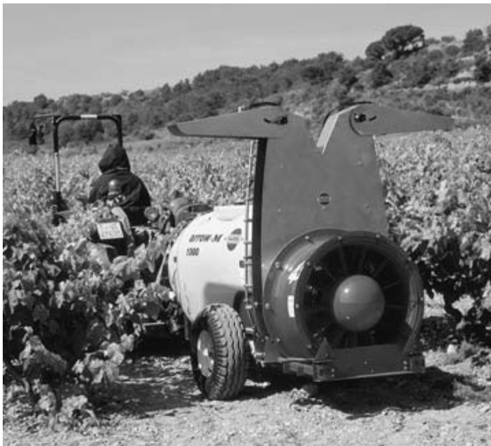
Fig. 3.4 Air-assisted sprayers for bush and tree crops. (a) Axial fan sprayer in apples; (b) in vines.
