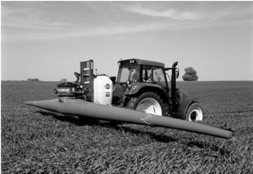
Fig. 3.3 Air-assisted boom sprayer provides a downwardly directed flow of air into the crop canopy.
