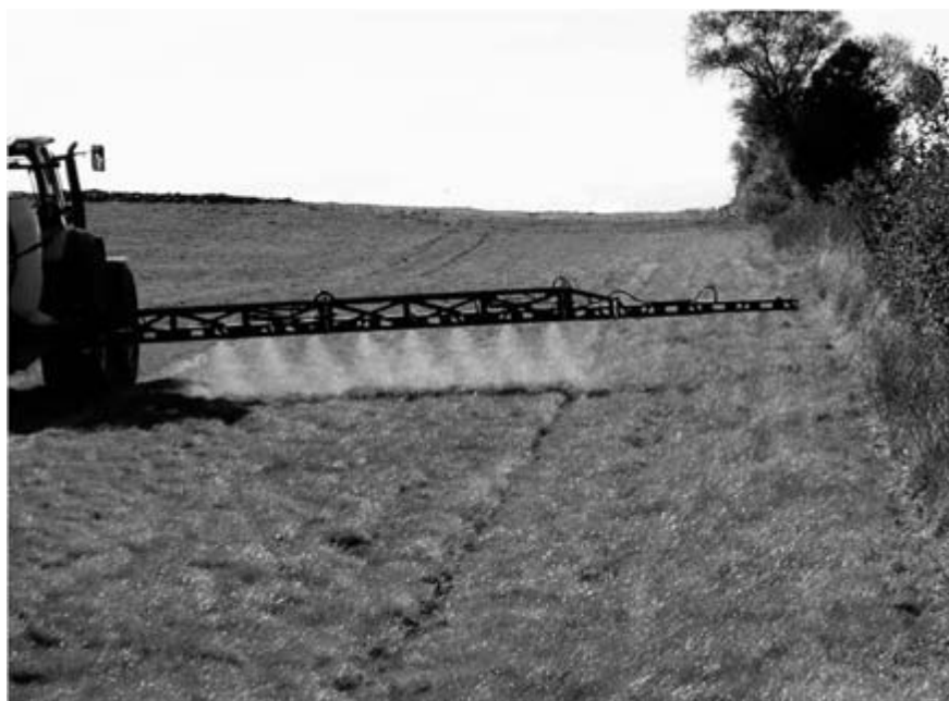
Fig. 6.3 Avoiding spraying from nozzles at the edge of the boom in order to reduce drift of spray into the hedge (photograph Hardi International).
