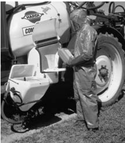
Fig. 4.1 Operating a sprayer. (a) Checking nozzle output with water; (b) examining nozzle calibration chart; (c) adjusting sprayer; (d) measuring pesticide. (Continued.)
