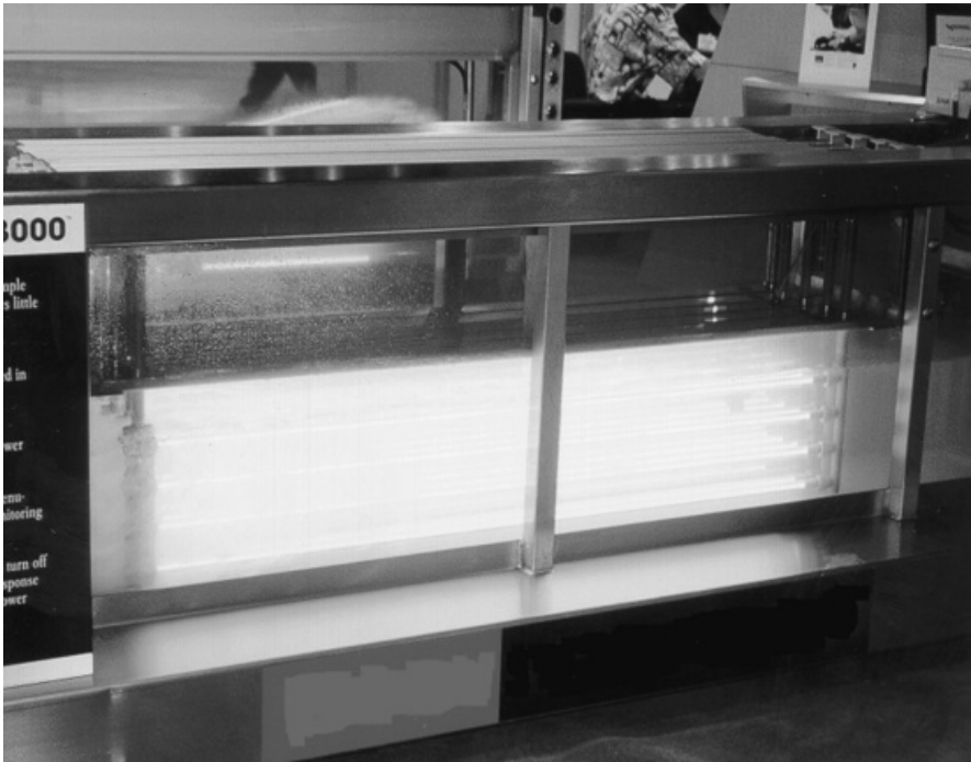
FIGURE 9.8 Horizontal lamps in a UV disinfection unit. The other potential configuration is with vertical lamps. In both cases, the flow is along the length of the lamps.
