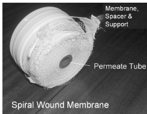
FIGURE 13.1 Partially disassembled spiral wound membrane. 1 Note: Mesh and backing to membrane.
