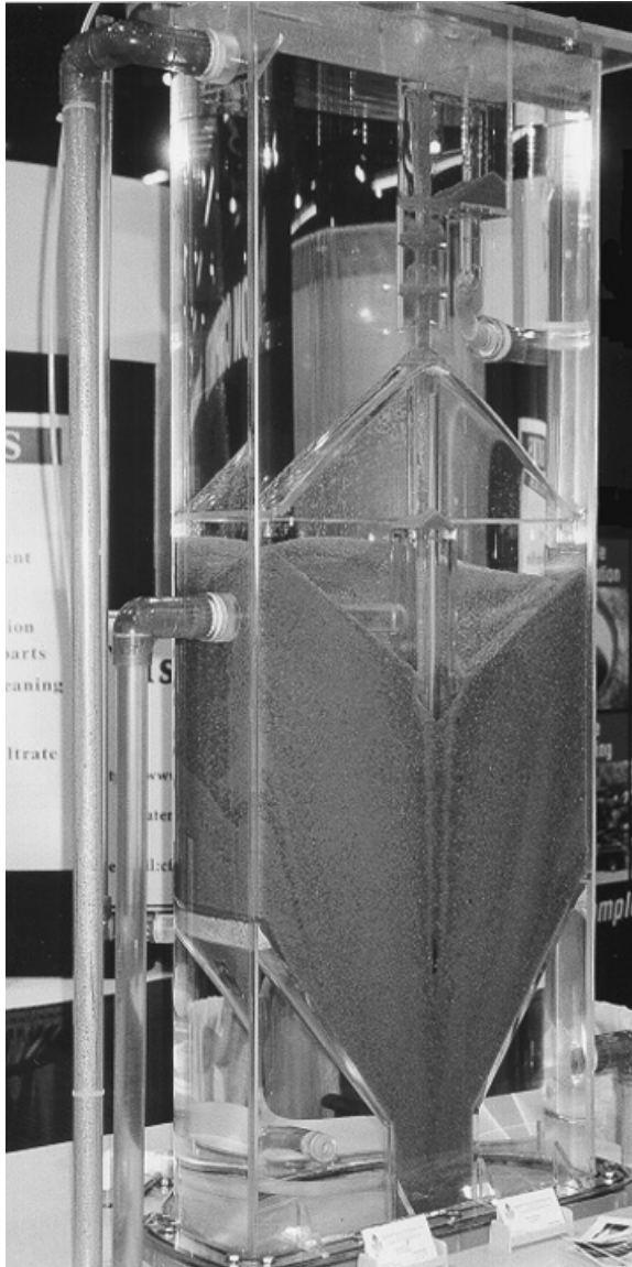
FIGURE 8.7 Cutaway view of a self cleaning sand filter.
