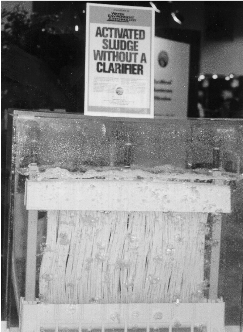
FIGURE 13.4 Spaghetti strand membrane clarifier in operation (taken at WEFTEC 2003).
