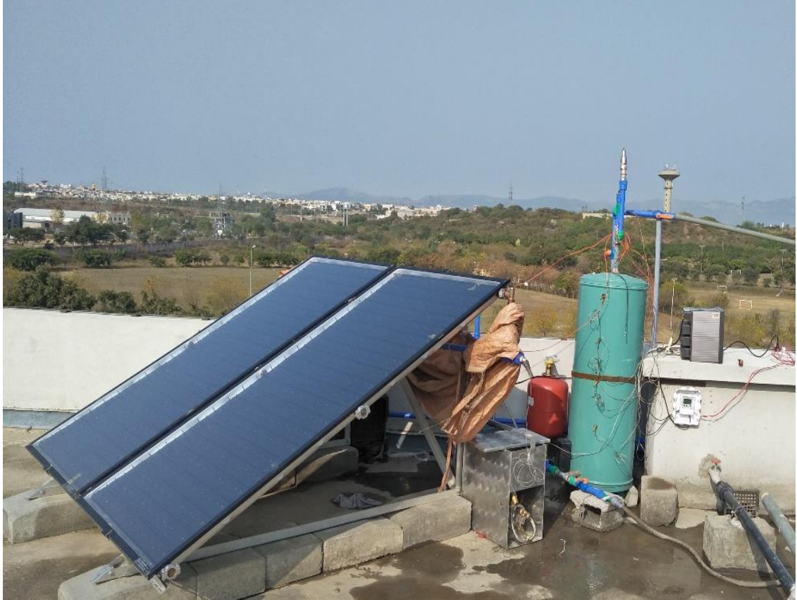
Figure 3.3 Experimental setup of evacuated flat plate collector model
