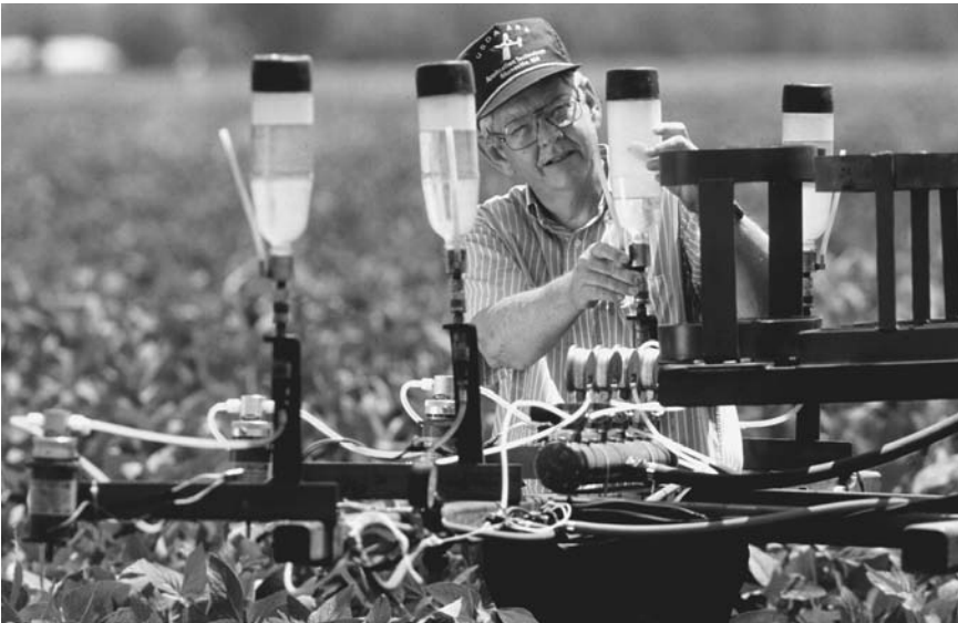
This ultra-low-volume herbicide applicator developed by plant physiologists is intended to reduce the use of agricultural chemicals. (Courtesy of the Agricultural Research Service, U.S. Department of Agriculture)
