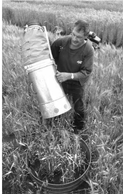
Sampling the insect population in an Iowa wheat field with a vacuum sampler (Courtesy of the Agricultural Research Service, U.S. Department of Agriculture)
