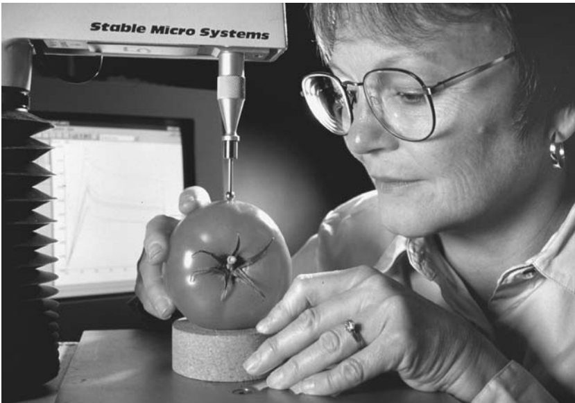
Tomato being tested for firmness (Courtesy of the Agricultural Research Service, U.S. Department of Agriculture)
