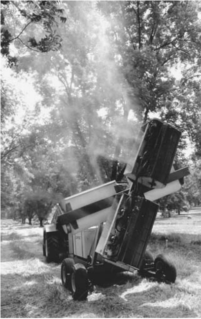
A newly designed insecticide fogger for use with orchard crops. It provides superior coverage of the treetops while using as little as one-third the amount of chemical. (Courtesy of the Agricultural Research Service, U.S. Department of Agriculture)
