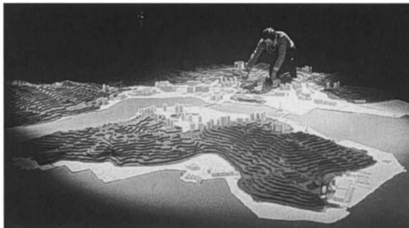
Figure 6.15 Wind tunnel model (photograph courtesy of BMT Fluid Dynamics, 1999)
