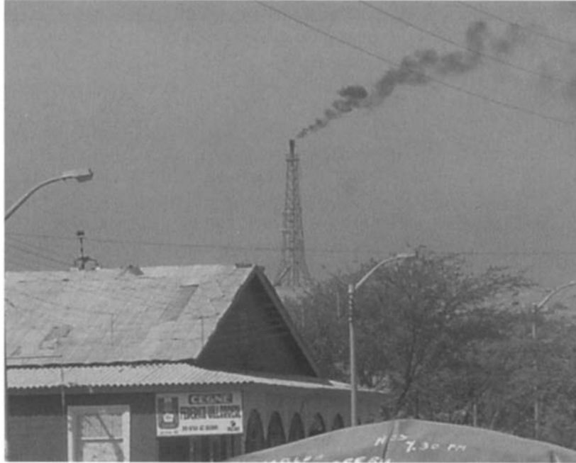
Figure 8.8 Flaring operations at an oil and gas terminal in Peru (courtesy of Cordah Limited)
