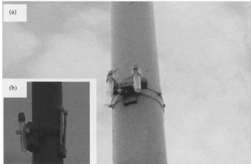
Figure 5.1 NO 2 and benzene diffusion tubes at a streetside location (courtesy of (a) Scottish Environment Protection Agency and (b) Environmental Health Department, Falkirk Council)
