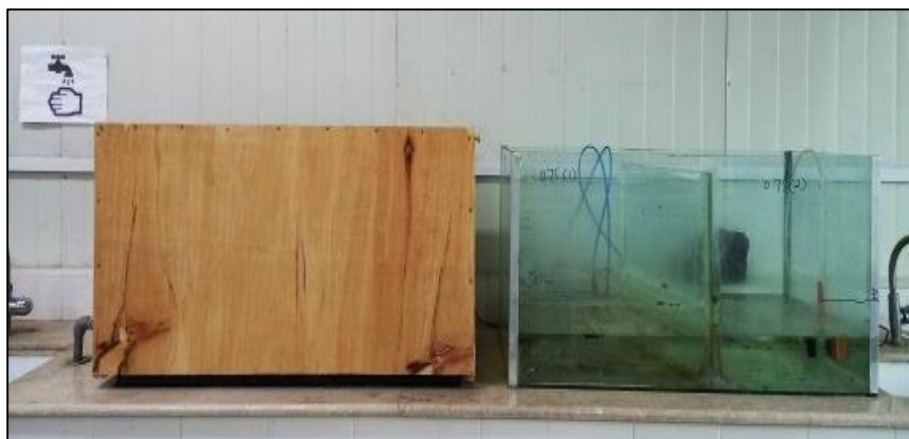
Figure 3.14 Experimental tank covered with wooden box
