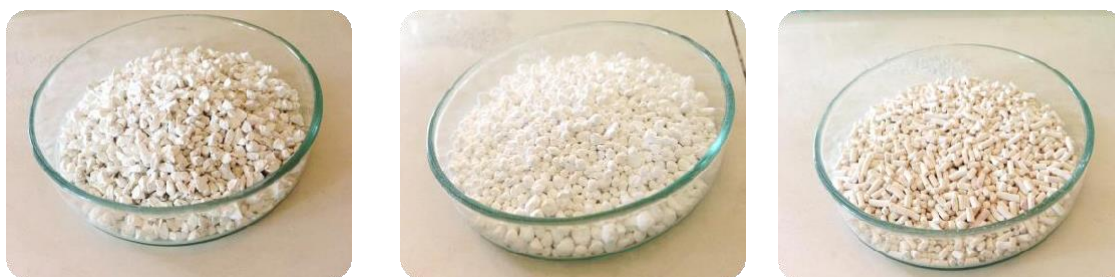
Figure 3.2 CaO, MgO and HZSM-5 catalyst
