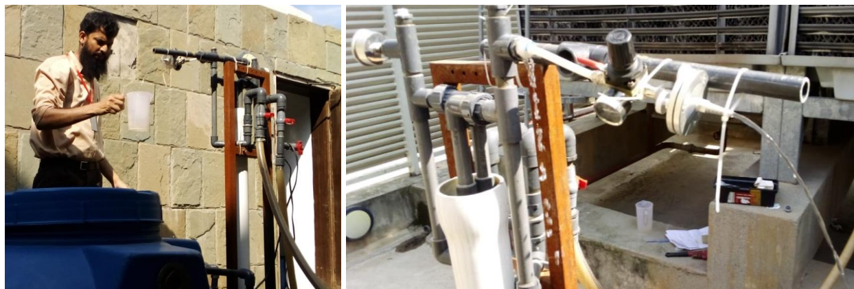
Figure 19: SDI Testing snapshot at CTBD stream
