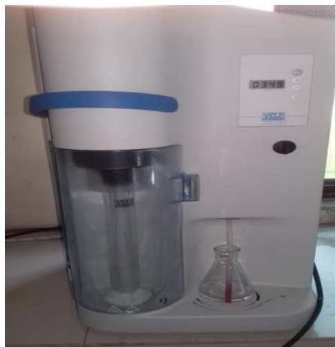
Figure 10: TKN distillation assembly unit
