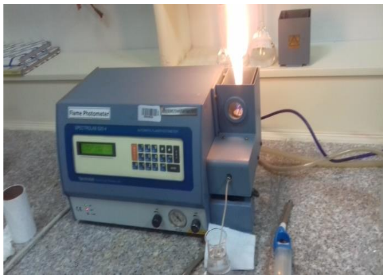
Figure 11: Flame photometer used for measurement of the K content
