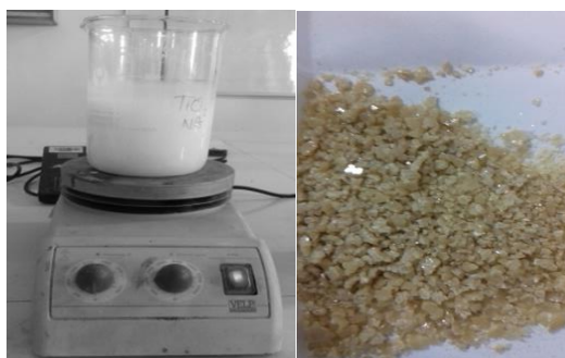
Figure 3: Synthesis of nTiO 2 through liquid impregnation method
