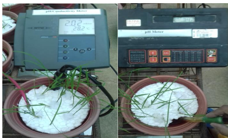
Figure 6: Measurement of the Hoagland nutrients solution's pH and EC
