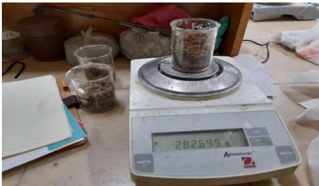
Figure 3-9 Measurement of Moisture Content Through Oven Dry Method
