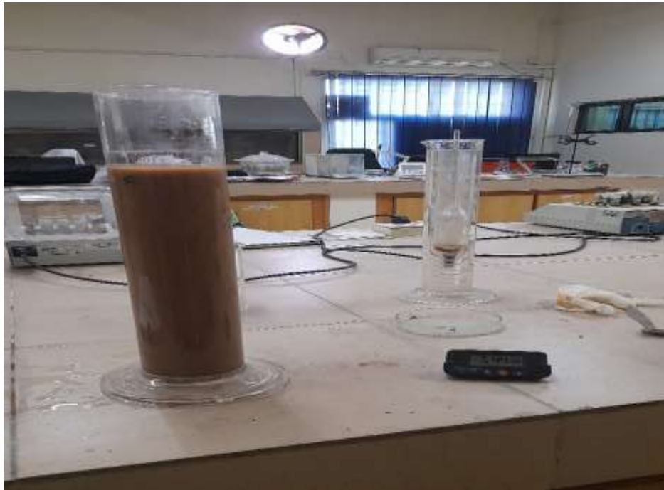
Figure 3-13 Hydrometer Analysis Test Conducted on Sample Taken from NBS Lawn
