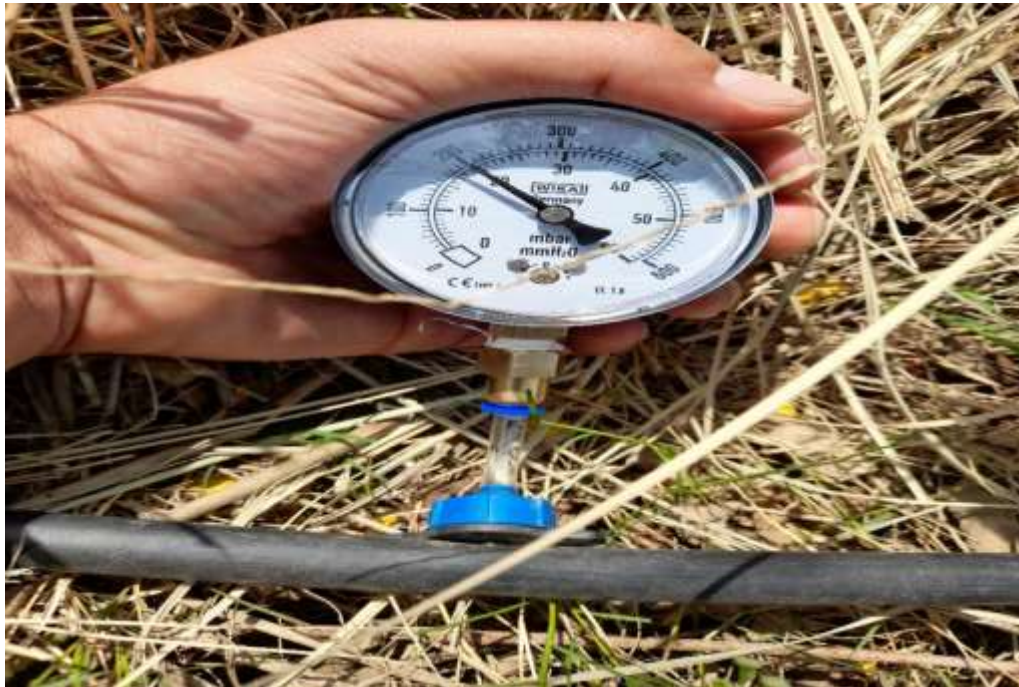
Figure 3-7 Measurement of Drippers Pressure at NBS
