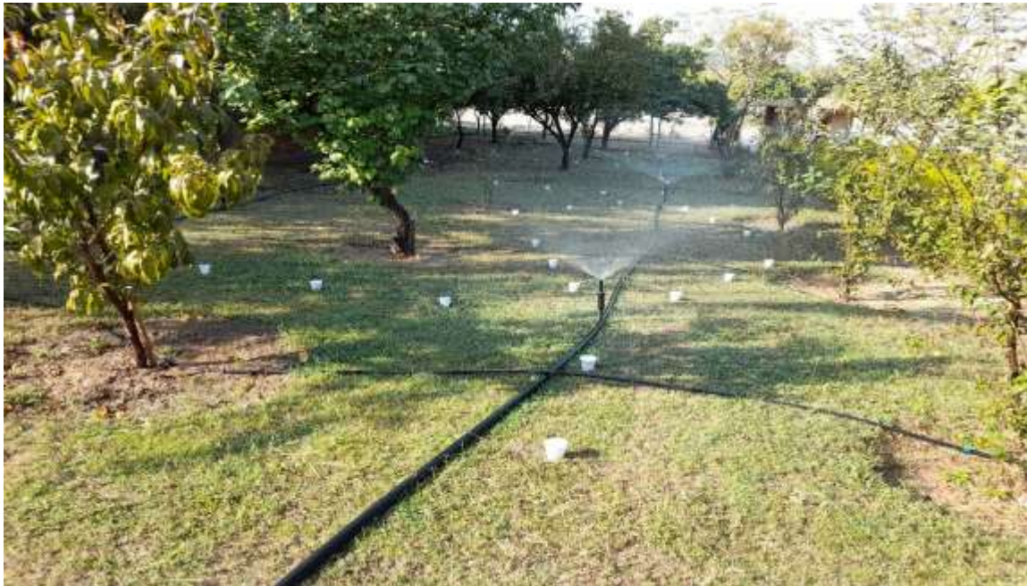
Figure 3-10 Measurement of Distribution Uniformity and Precipitation rate of Sprinklers
