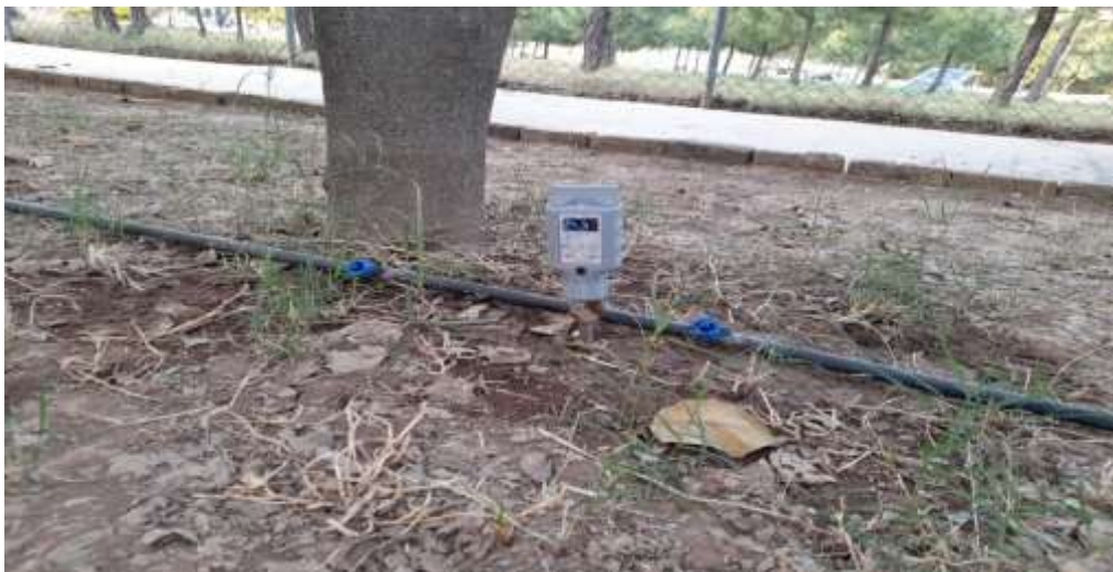
Figure 3-8 Measurement of Moisture Content Through Tensiometer
