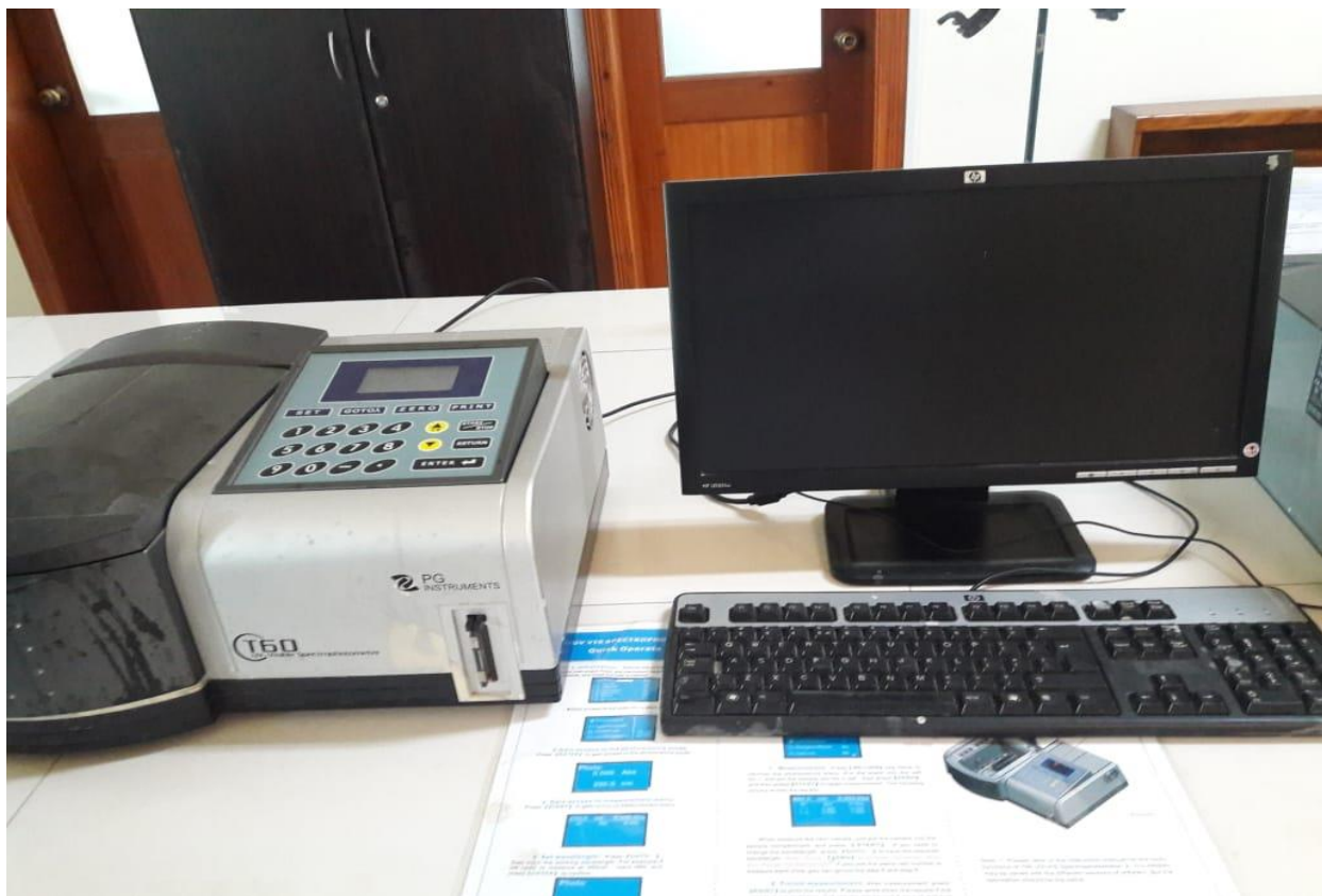
Figure 3.6: UV Spectrophotometer for the Quantitative Determination of Cr (VI)
