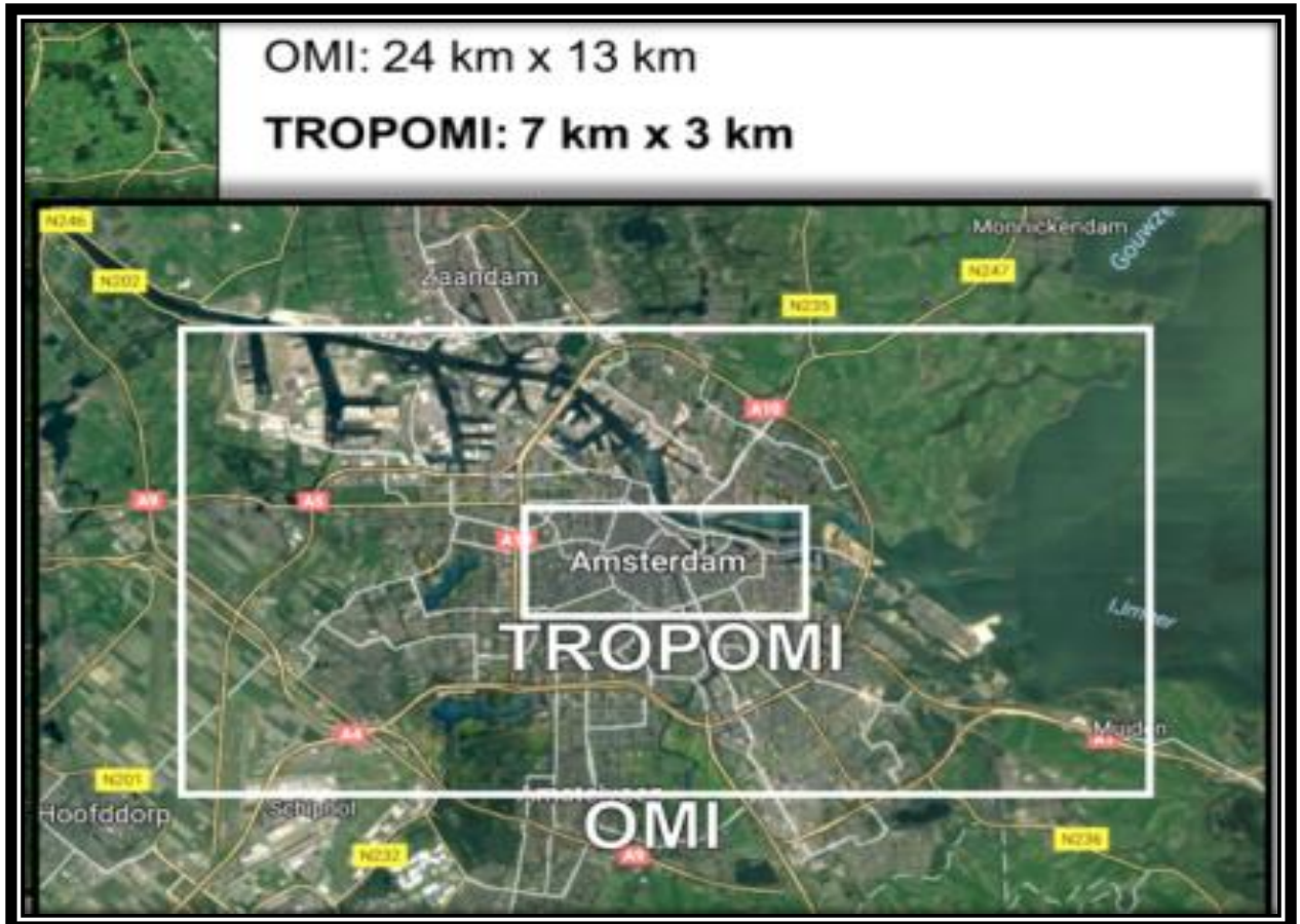
Figure 3. 2 Comparison of TROPOMI and OMI instruments (Source: https://www.tudelft.nl/en/2017/citg/grs/what-makes-tropomi-special/ )
