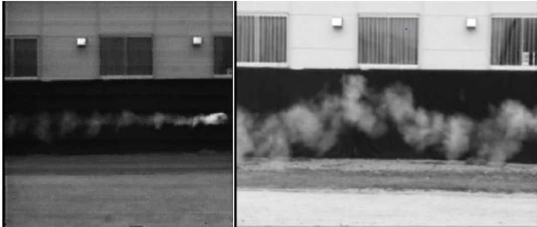
Figure 2.2 Wide-angle view of the vortex pathway for a non-rotating ball [11, 12]
