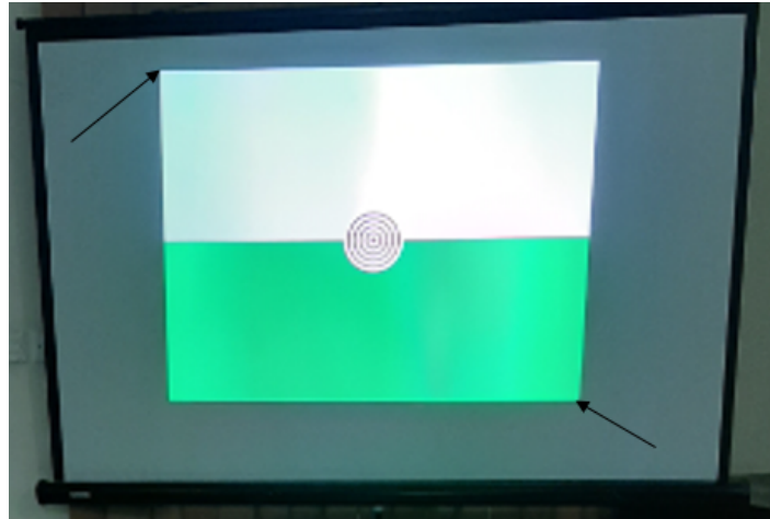
Figure 3.4: Calibration to specify the screen area by clicking top left and bottom right corner
