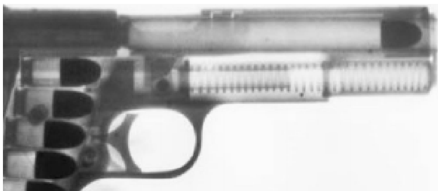
Figure 2.4: X-Ray image of bullet travel inside the barrel [23]
