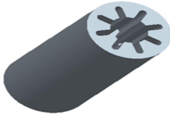
Figure 4.1 (a) Initial finocyl grain model
