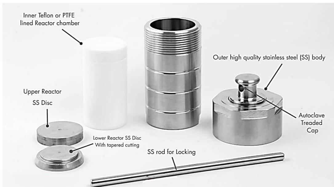
Figure 3.1 Autoclave used for the hydrothermal synthesis technique.
