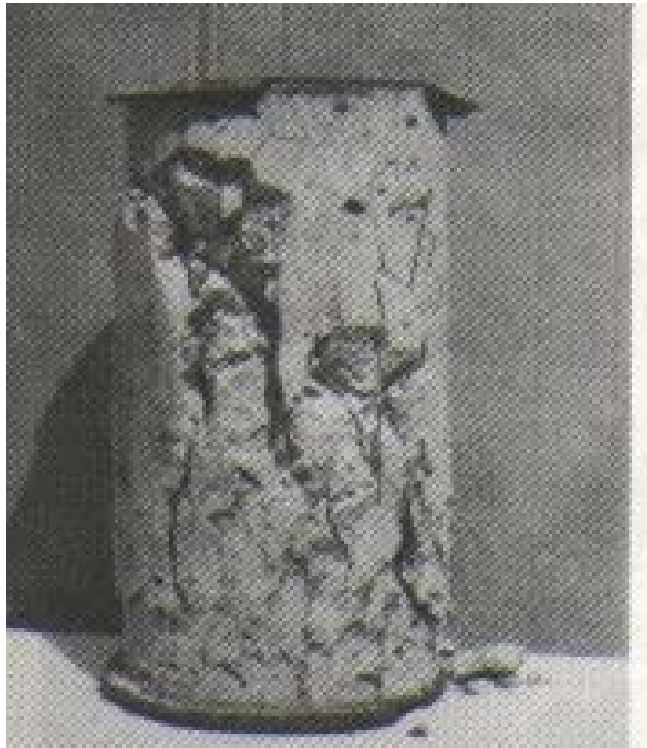
Compression Failure Without Silica fume
