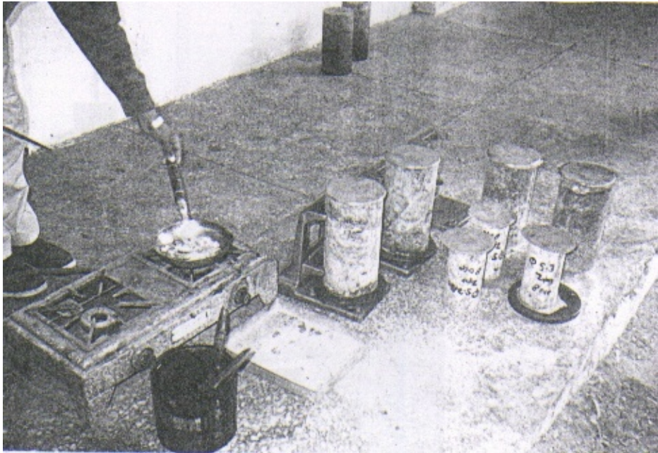
Capping in Progress
