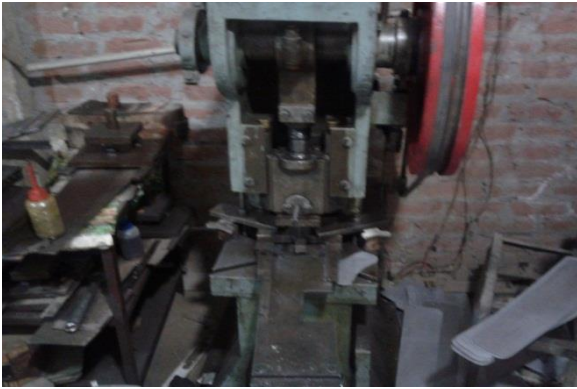
(a) Blade drilling machine
