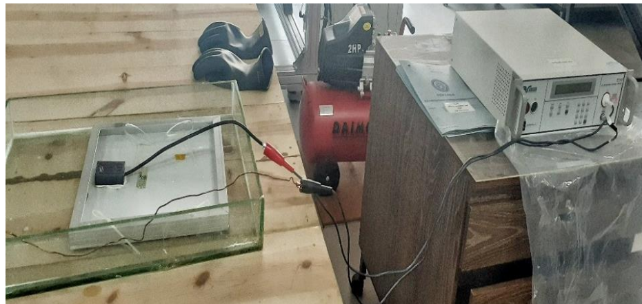
Figure 3.7 Wet Leakage current test setup showing module under test.
