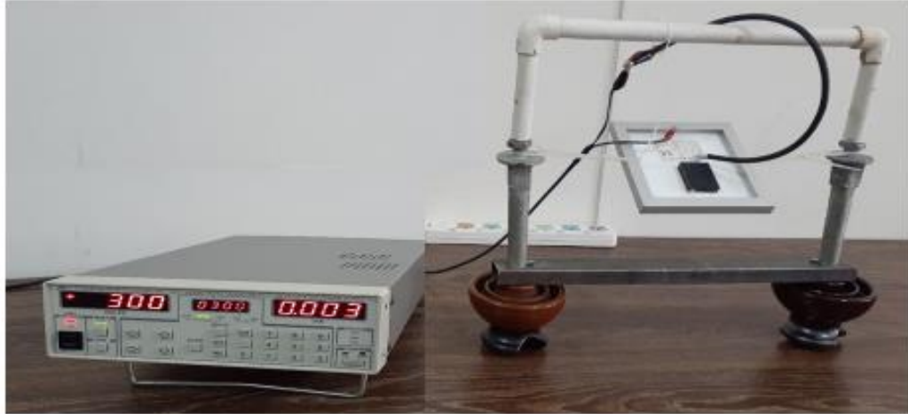
Figure 3.10 Outdoor application of high voltages on module using Stanford DC power supply.
