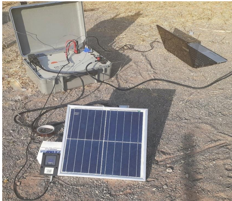
Figure 3.4 Daystar IV Curve Tracing Setup showing module during test.
