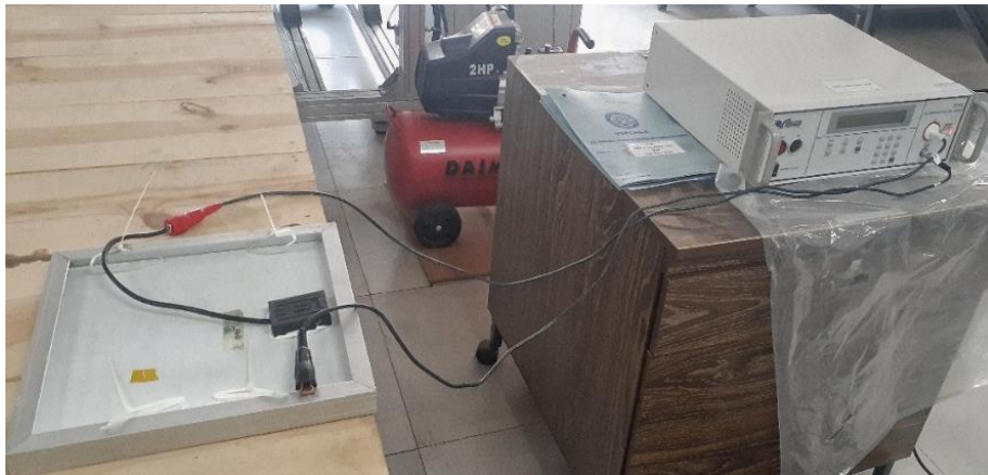
Figure 3.6 Dry Insulation test setup showing module under test.
