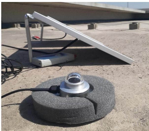
Figure 3.2 Stabilization of Modules by sunlight exposure.
