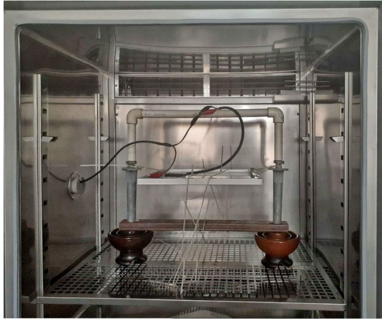
Figure 3.9 Insulation Stand for holding PV module inside environmental chamber.
