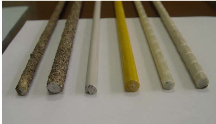
Fig. 2.1. GFRP bars of various diameters and surface types
