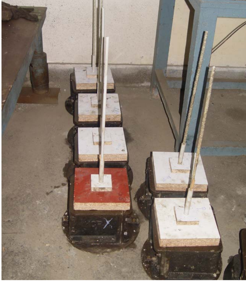
Fig. 3.1. GFRP rebars cast in concrete cubes with bar alignment jig.
