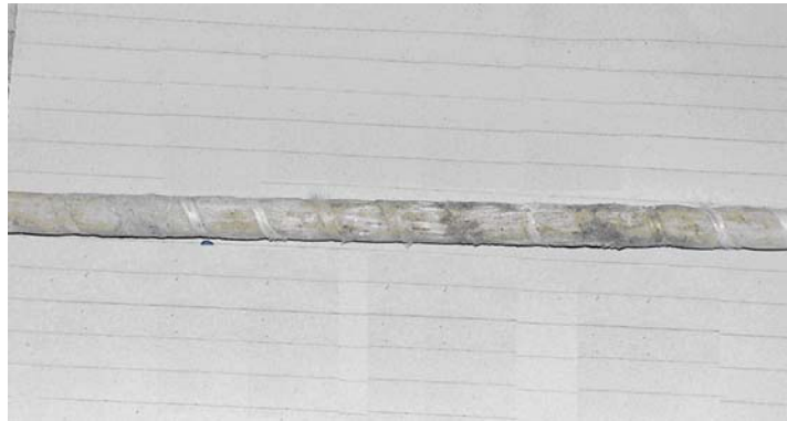
Fig. 4.1. Damage to the deformed GFRP bar after pullout
