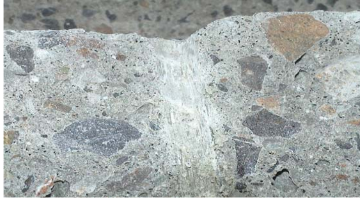
Fig. 4.3. Cross-section of concrete block showing crushed resin and chopped glass fiber remains
