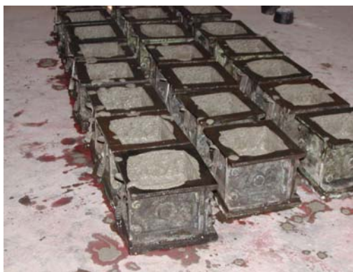
Fig. 5. 6-Inch cube molds
