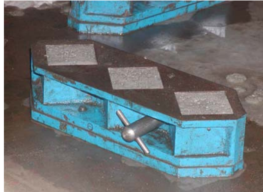
Fig. 2. 2-Inch cube molds
