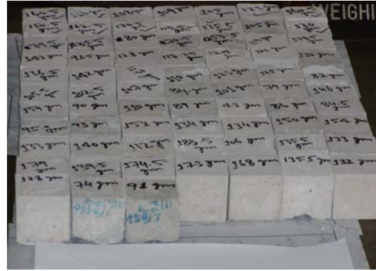
Fig. 2. Specimens for water absorption test
