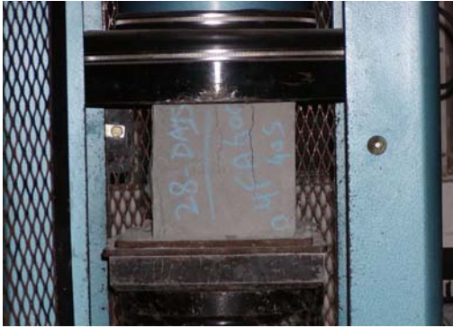
Fig. 1. 28-days cracking failure
