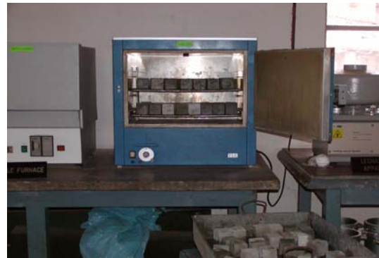
Fig. 4. Oven-drying of specimens
