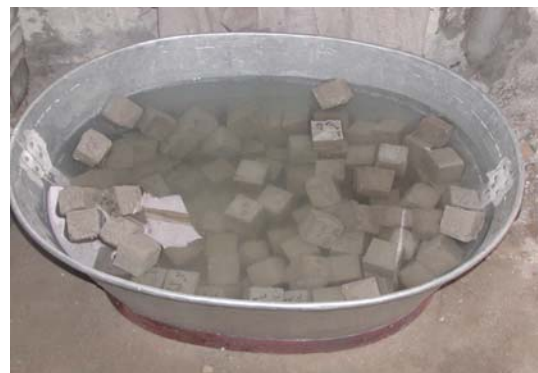
Fig. 6. Curing of samples in progress
