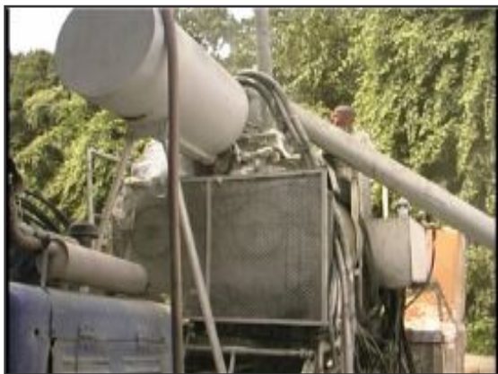
Fig. 1.1. Equipment set for production of Foam concrete (Litebuilt 2005)
