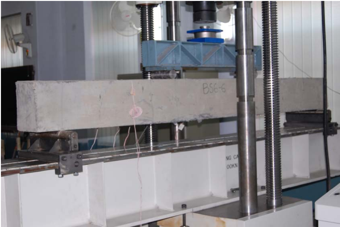
Fig 4.18 (a) - Cracking pattern BS 6-6
