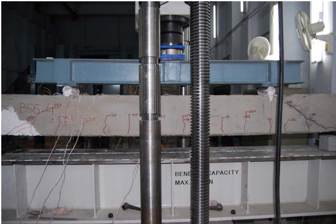
Fig 4.16 - Cracking pattern BS 6-4
