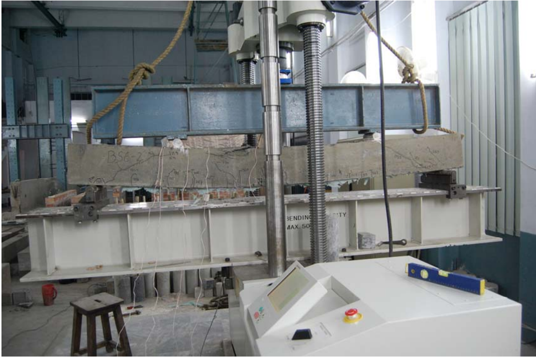
Fig 4.14 (a) - Cracking pattern BS 6-2
