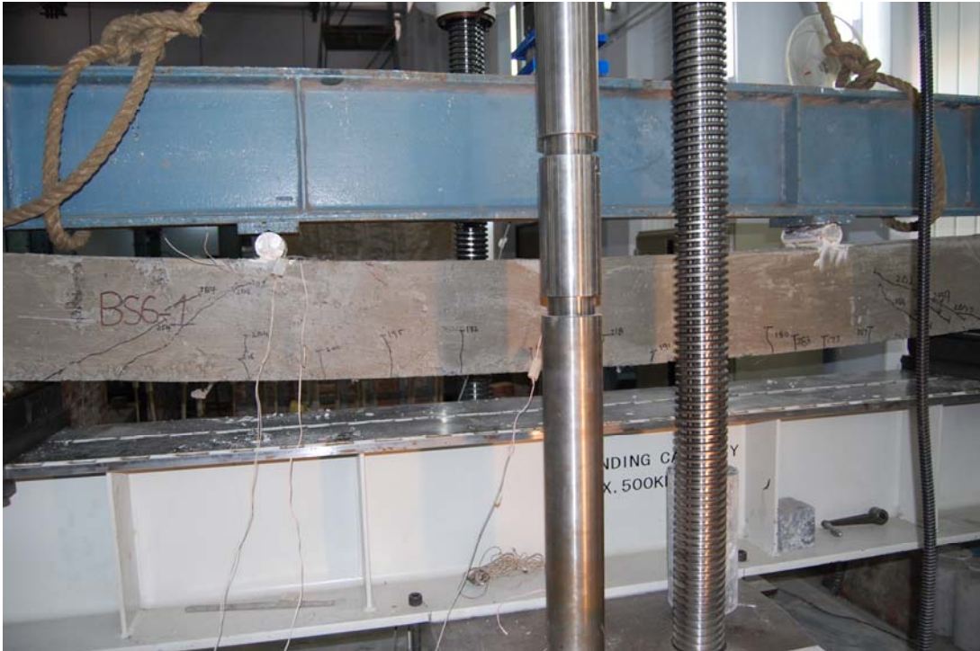
Fig 4.13 (a) - Cracking pattern BS 6-1
