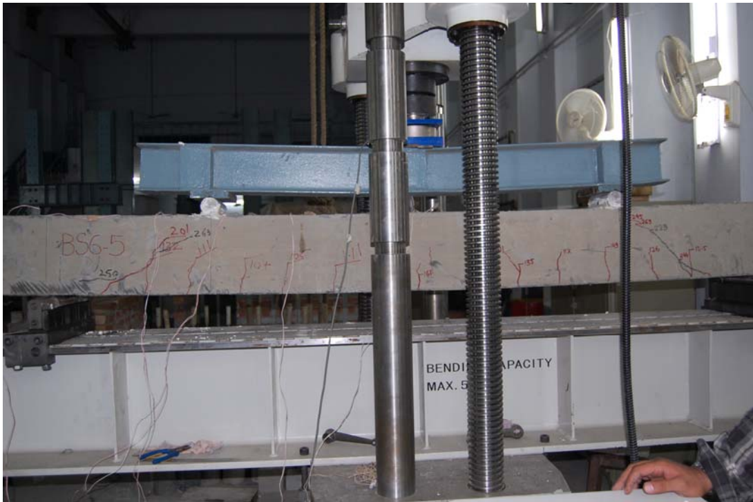
Fig 4.17 - Cracking pattern BS 6-5
