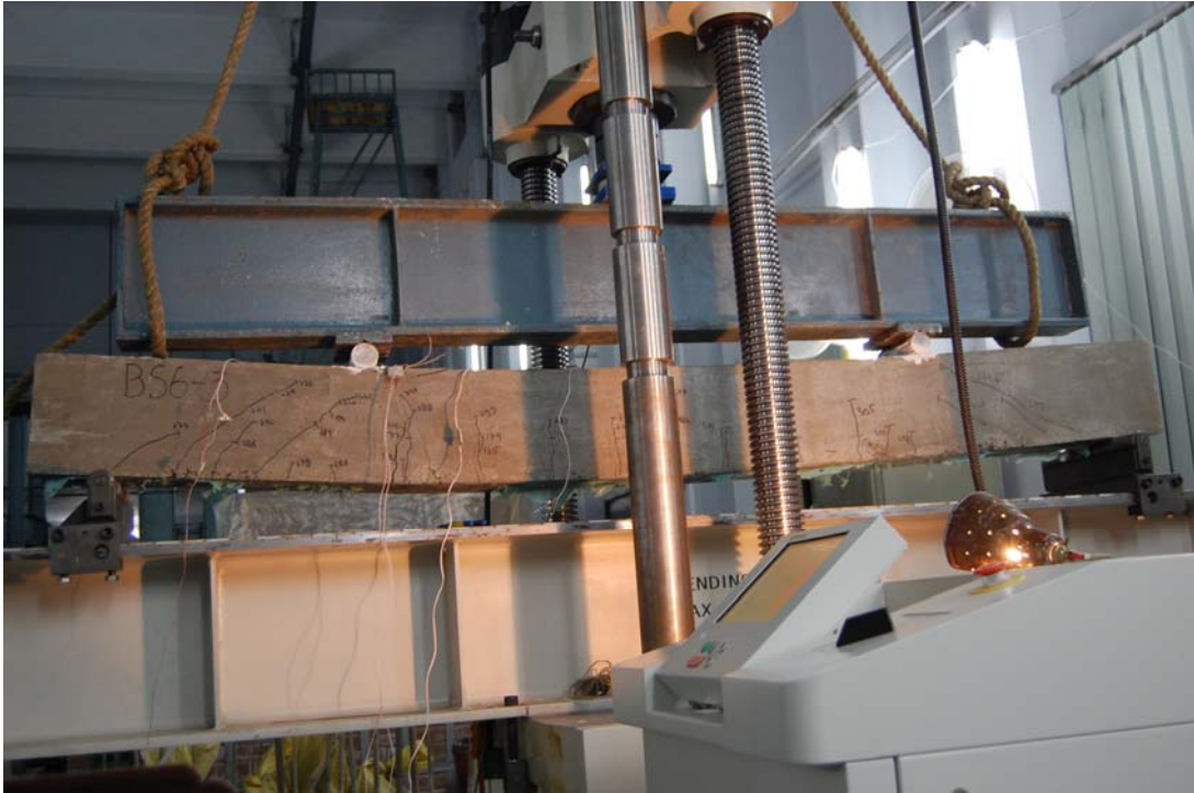
Fig 4.15 - Cracking pattern BS 6-3
