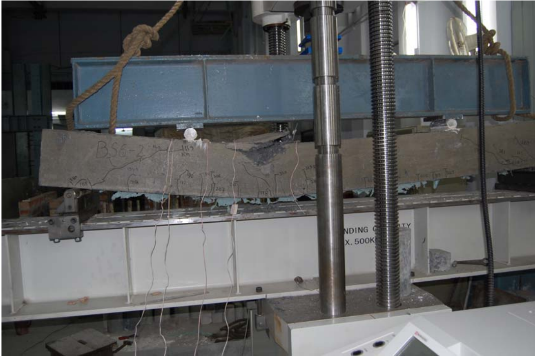
Fig 4.14 (b) - Cracking pattern BS 6-2
