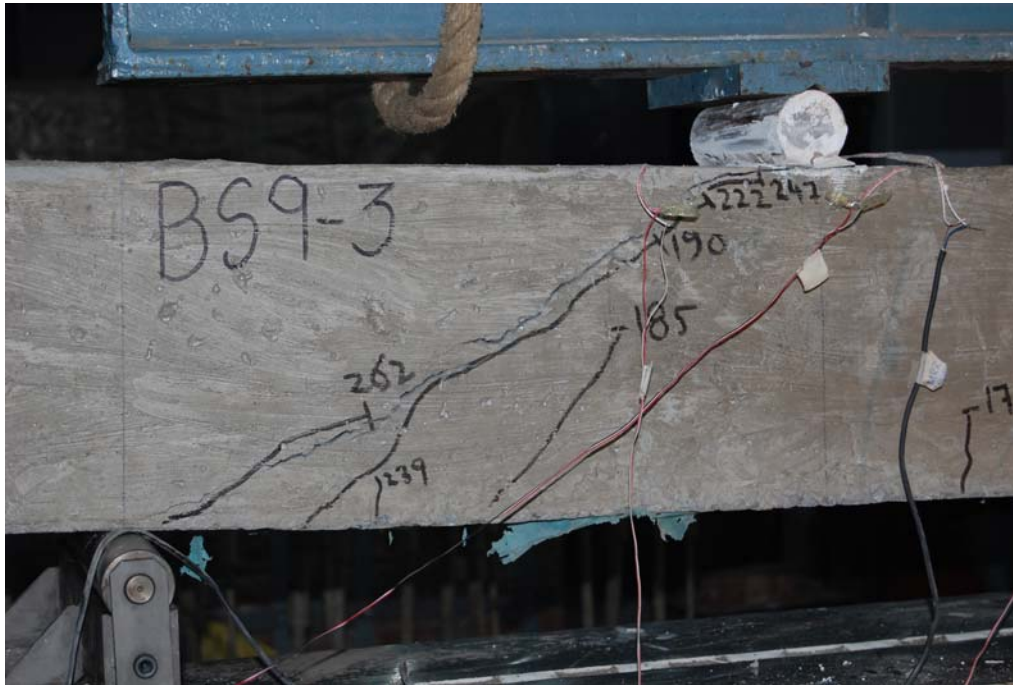
Fig 4.14 (a) Cracking pattern BS 9-3
