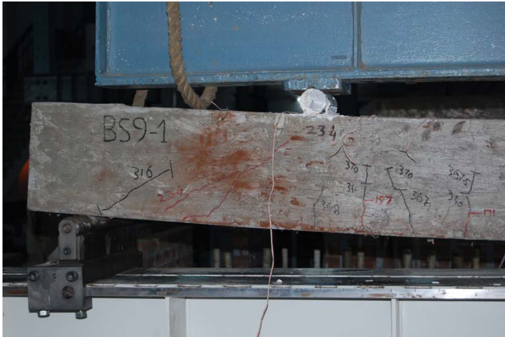
Fig 4.12 (a) Cracking pattern BS 9-1
