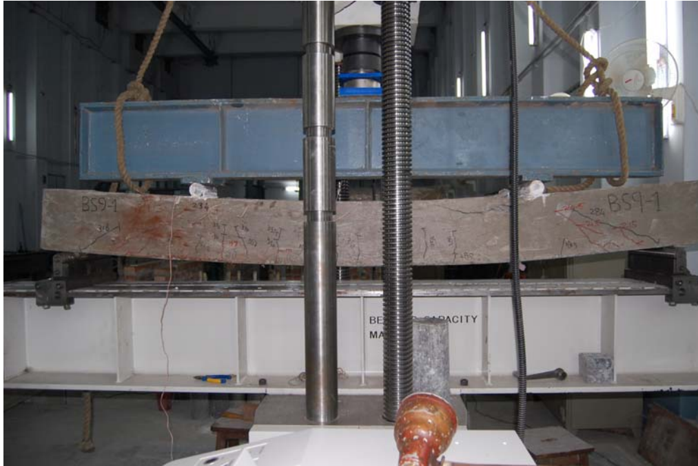
Fig 4.12 (b) Cracking pattern BS 9-1
