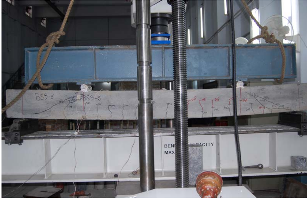
Fig 4.17 (a) Cracking pattern BS 9-6
