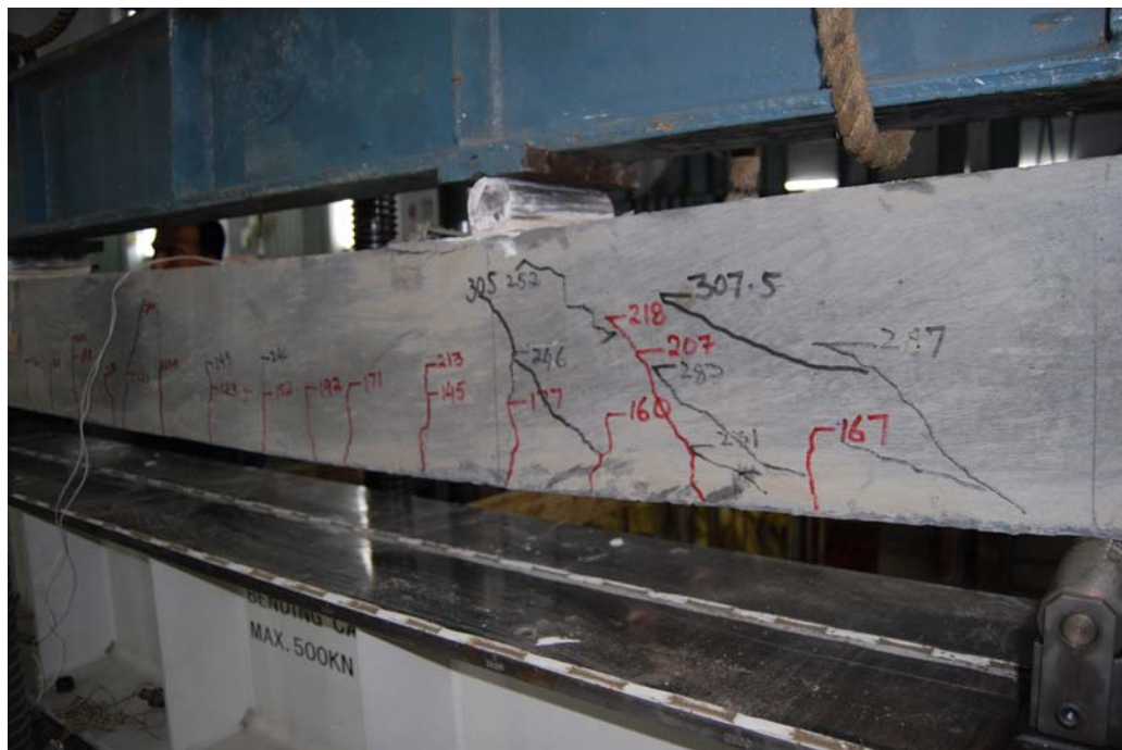
Fig 4.15 (b) Cracking pattern BS 9-4
