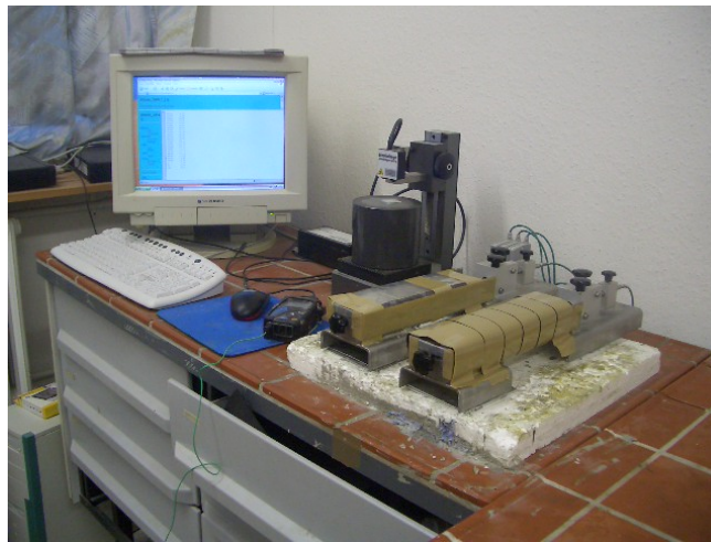
Fig 3.1 German modified shrinkage channel apparatus
