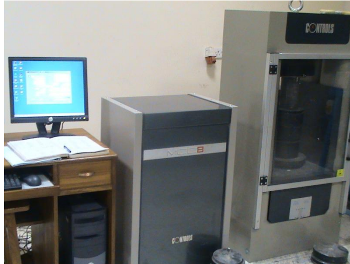
Figure 3.3: A Servo-hydraulic Computer Controlled Compression Testing Machine
