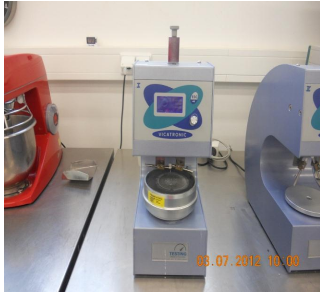
Fig. 3.1 Automatic VICAT apparatus used to determine Initial & Final setting times
