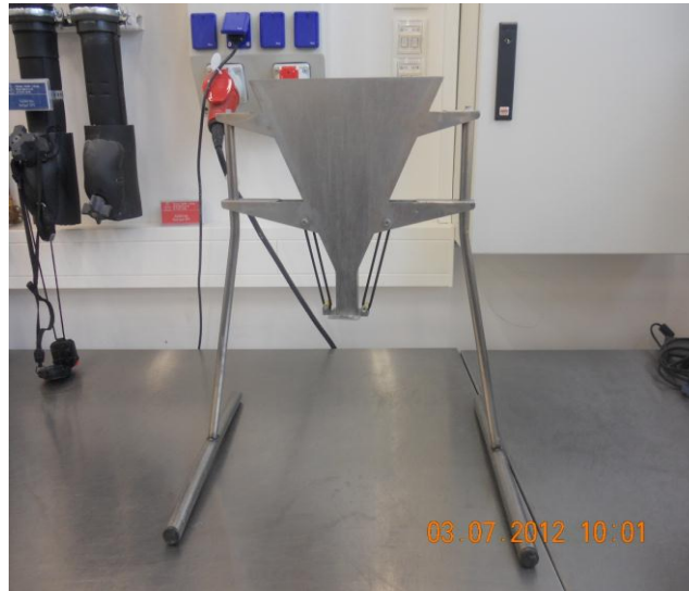
Fig. 3.3 V-funnel apparatus used for determining flow times of SCM formulations.
