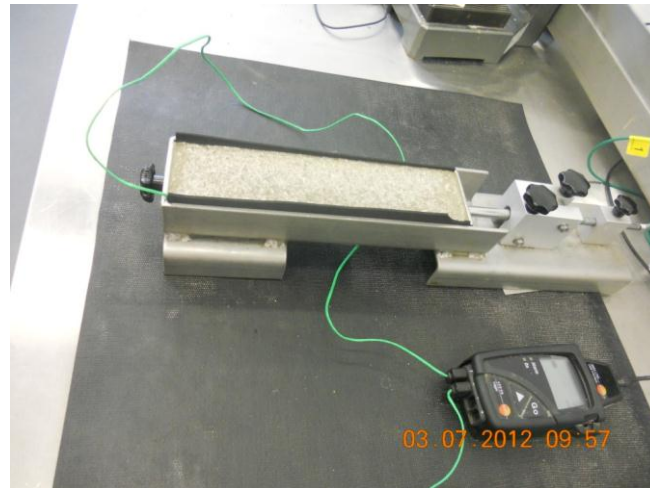
Fig. 3.6 Sensors of “Testo”, immersed in the fresh shrinkage sample
