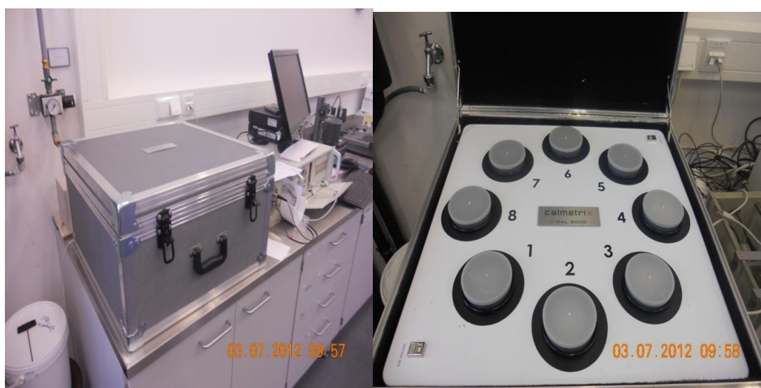
Fig. 3.5. Semi-adiabatic Calorimeter used for determining hydration kinetics.
