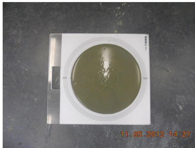
Fig. 3.2 Target spread of 30\pm 1 cms achieved using Hagermann cone.
