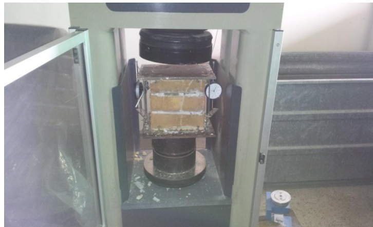
Figure 3.4: compression testing of brick masonry prisms
