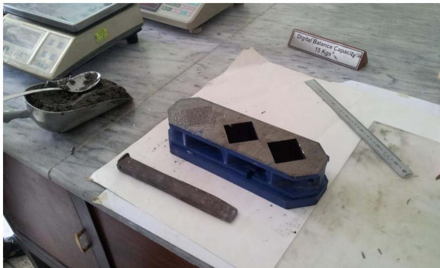
Figure 3.2: Preparation of 2 in mortar cubes.
