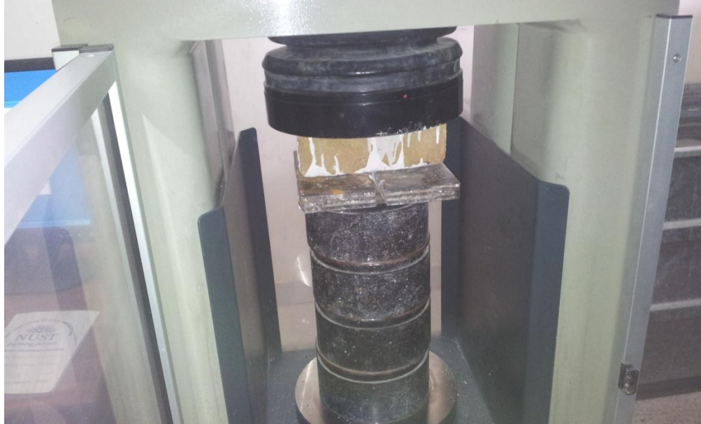
Figure 3.1: compressive strength test of brick masonry unit.
