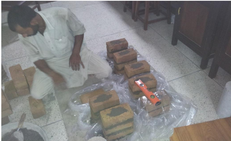
Figure 3.3: Preparation of brick masonry prisms.
