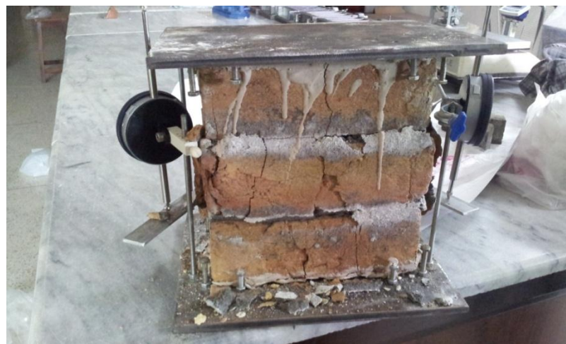
Figure 3.5: Brick masonry prism in testing rig with displacement gauges.
