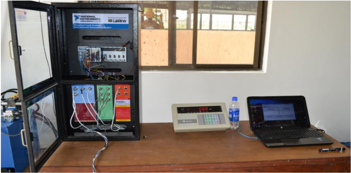
Figure 4.1: Structural Load Analysis and Automation System
