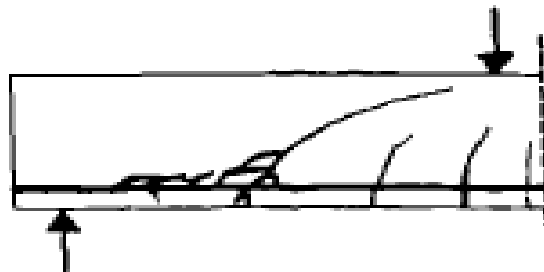
Figure 2-7 : Shear tension failure
