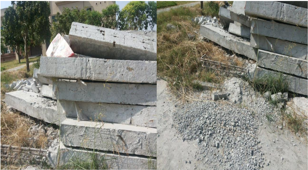
(a) Beams used for acquiring recycled aggregates
