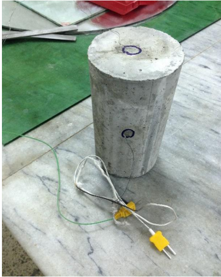
Thermocouple being embedded in concrete cylinder
