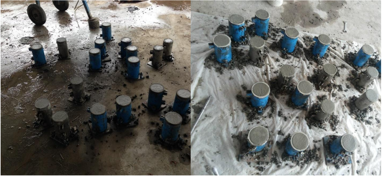
Fig. 3.5. Casting of specimens
