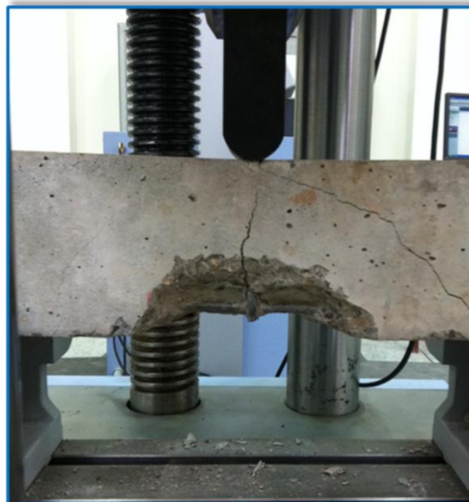
Fig.3.4 A failed Control Beam
