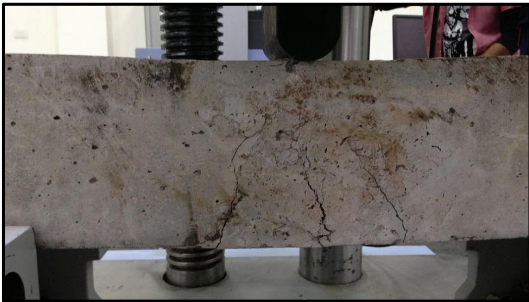
Fig.3.5 A failed FRC Repaired Beam
