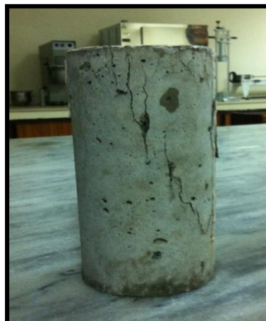
Fig. 2.3 A failed specimen after compressive strength test
