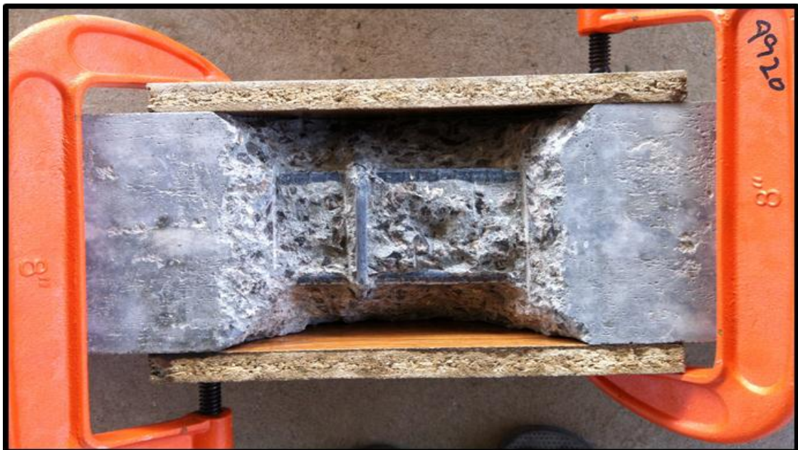
Fig. 3.1 A damage induced Beam with formwork
