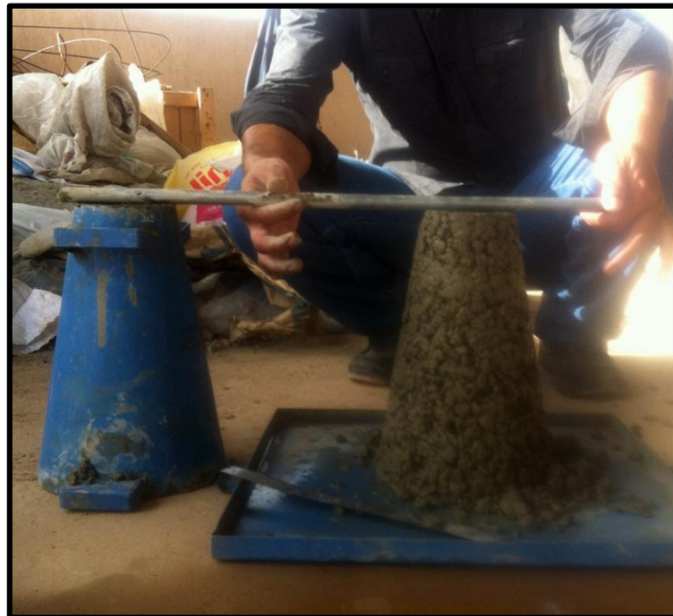
Fig. 2.2 Slump Test showing True Slump
