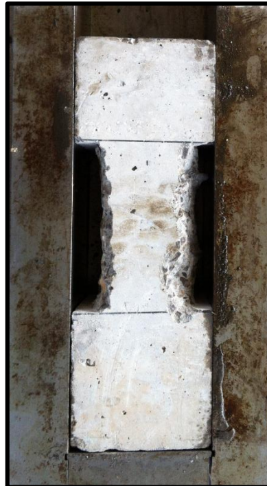
Fig. 3.2 A damage induced Column with formwork
