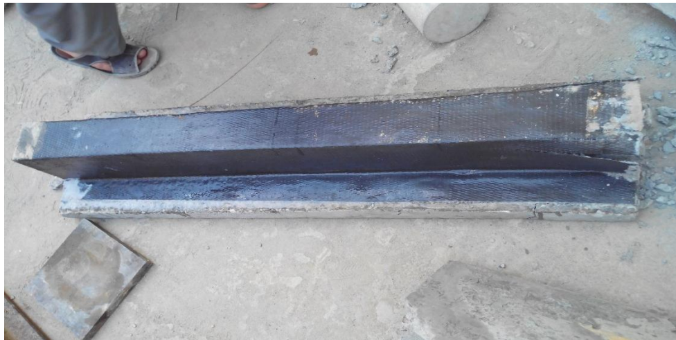
Figure 3.8: Failure pattern of BEAM3
