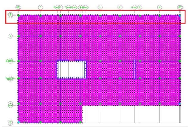
Grid 9 has nine columns named as 9B, 9C, 9E, 9H, 9J, 9K, 9M, 9N and 9O. Beams are shown between these columns in blue colour and their design can be seen also. There are total 8 beams provided in this grid as shown.
