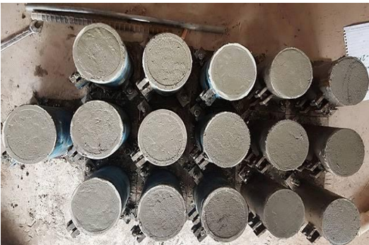
Figure 3.8: Casting of 4x8" samples
