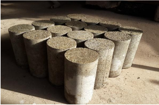
Figure 3.9: Samples casted for the compression and healing analysis
