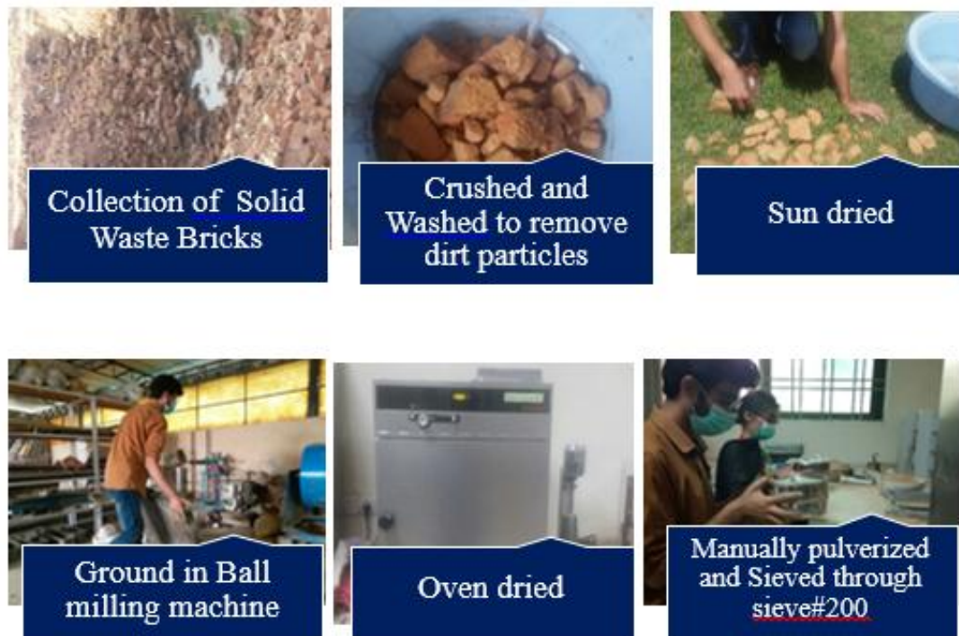
Figure 3.1 Brick powder preparation
