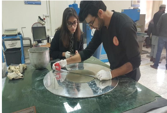
Figure 4.3 Hagerman mini cone apparatus for SP demand
