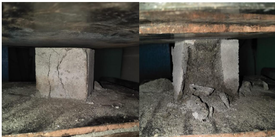
Figure 12: Compressive testing on samples
