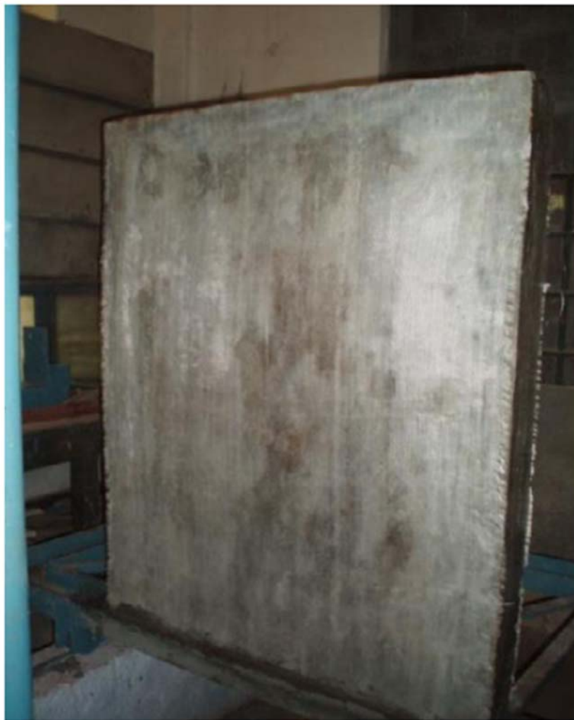
Figure 2.9. GFRP wrapped wall
