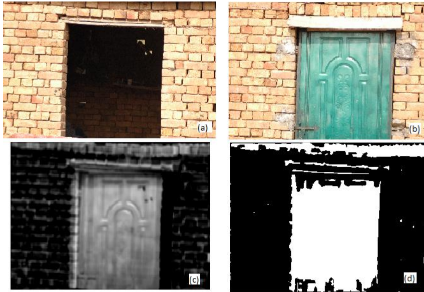
Figure 4.14 (a) Wall image at T=10, (b)Wall image at T=15 (c) Blurred Difference (d) Binary Door Location
