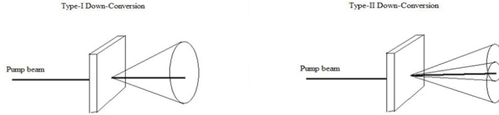
Figure 2.1: shows parametric down conversion process. Photons coming out of crystal form cones. In parametric down conversion type I both photons belonging to single pair appear on same cone with same polarization of both photons. In type II parametric down conversion photons produced as a result of down conversion appears in different cones with one photon having horizontal polarization and other with vertical polarization.
