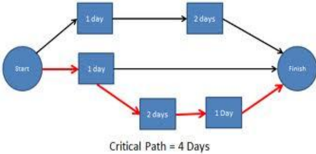
Figure 2.6 Critical Path Method Sample
