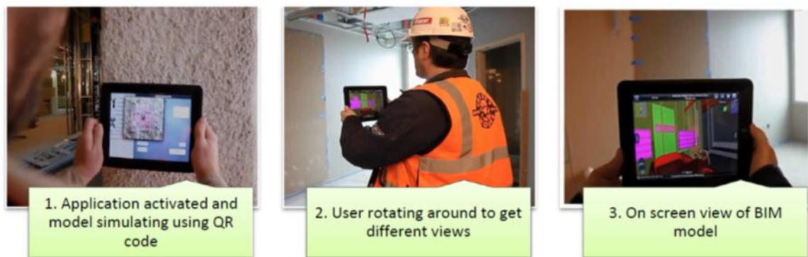
Figure 2-5 showing BIM Filed demo (BIM field,2013)
