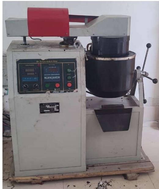
Figure 3-13: Mixing of Asphalt and Aggregate
