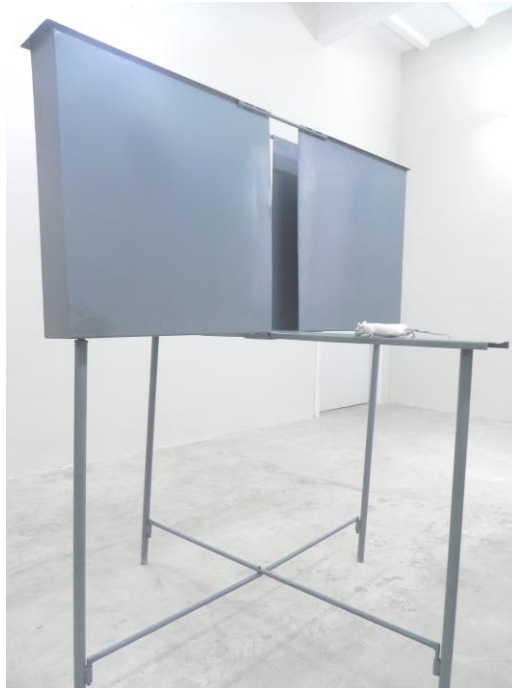
Figure 3.2: Elevated plus maze apparatus consisting of two open arms and two closed arms
