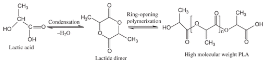
Figure 2.3: Polymerization of lactic acid. Adapted from ref.(Ahmed & Varshney, 2011)
