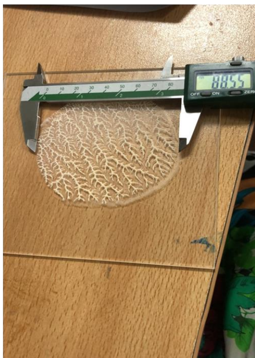
Figure 18: Spread Ability Measurement Using Vernier Caliper
