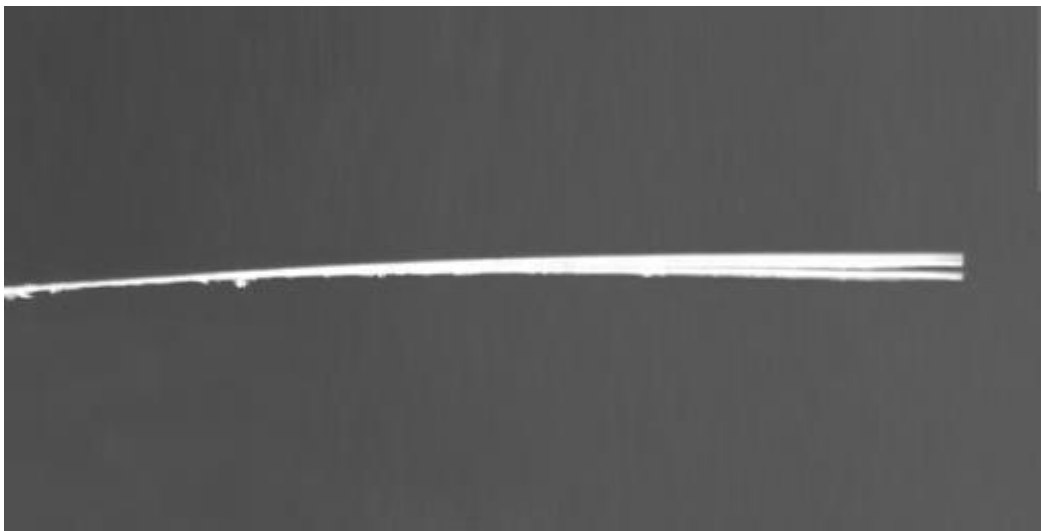
Figure 4.16 Stroboscopic image for amplitude of A/L= 0.02
