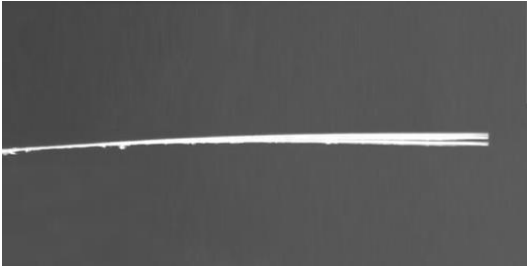
Figure 4.15 Stroboscopic image for amplitude of A/L= 0.028
